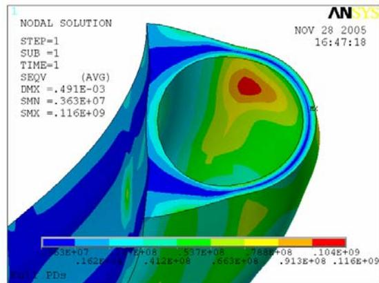
a) Compressive effect due to PDs.      b) Inner tube bending effect due to the thickness increase.
