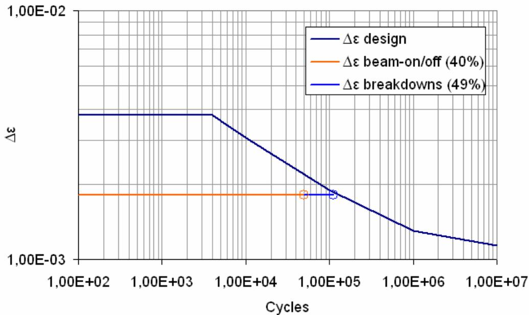
**Figure 13. Fatigue damage of 89% for beam-on beam-off and breakdown cycles at the worst loaded node of the neutralizer LEE.**
