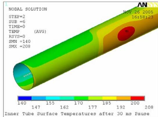
a) Body temperatures of CuCrZr-IG [°C].      b) Inner tube surface temperatures [°C].
