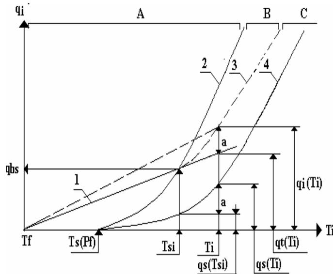
**Figure 1. Regions of heat transfer conditions in the tube channel [6],  $q_i(T_i)$  is heat flux. The regions are divided by the boundaries: 1) turbulent heat transfer boundary, 2) boundary of the surface boiling start-up, 3) boiling curve approximation in the forced coolant flow, 4) boiling curve for the saturated coolant flow.**
