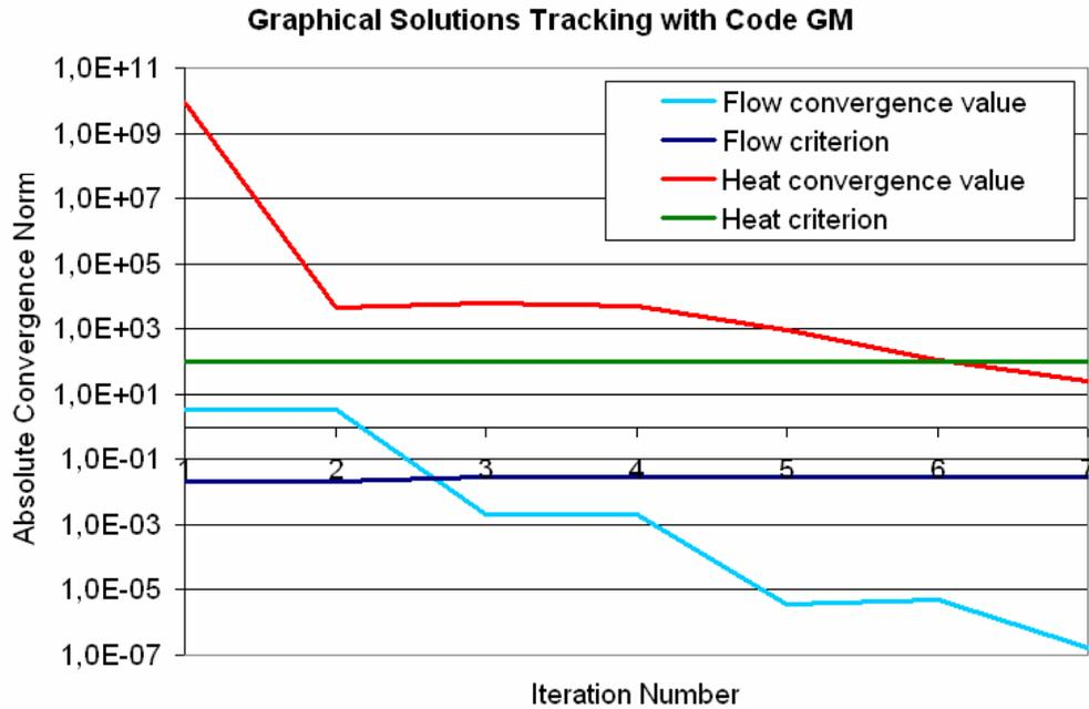
**Figure 4. Graphical solutions tracking for nonlinear analysis solved with code GM. 7 iterations to convergence.**
