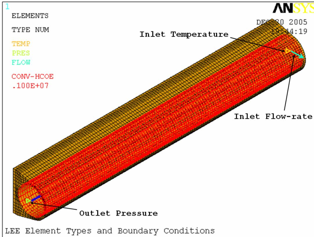
**Figure 2. Element types of the neutralizer LEE model. ■: 3-D solid thermal/structural elements. ■: coupled thermal-fluid pipe elements. ■: 3-D thermal surface elements. The constant heat transfer coefficient assigned before the solution is displayed. The applied boundary conditions are the inlet coolant temperature, inlet flow-rate, and outlet pressure.**
