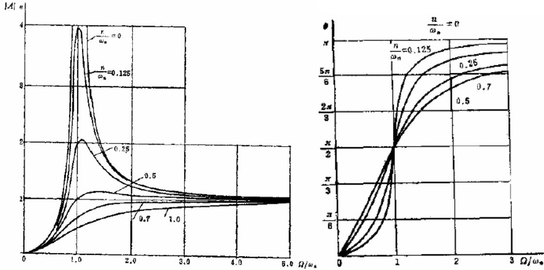
Figure 2. Synchronous Response Diagram [2]
