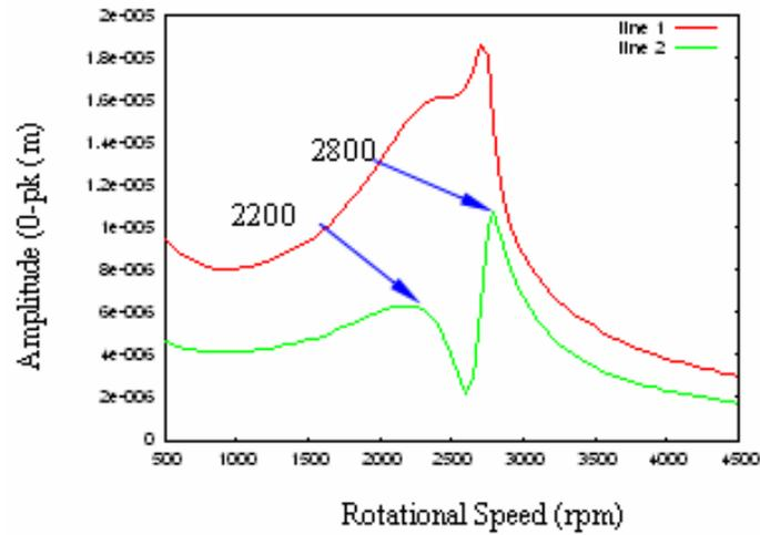
Figure 4. Unbalance Synchronous Response
