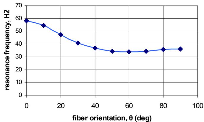
**Figure 8. Effect of fiber orientation on resonance frequency**
