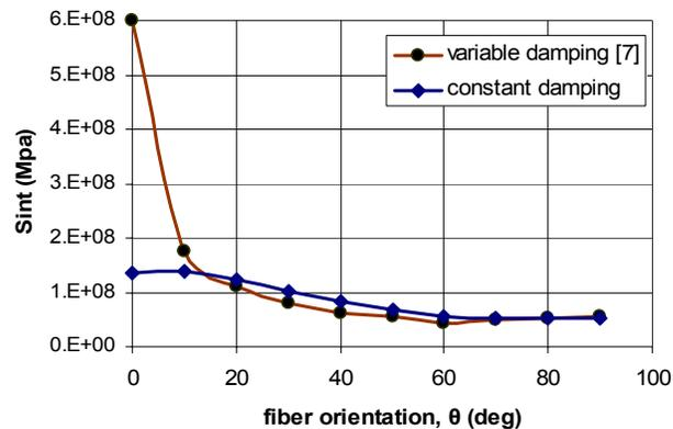
**Figure 7. Effect of fiber orientation on max stress intensity**
