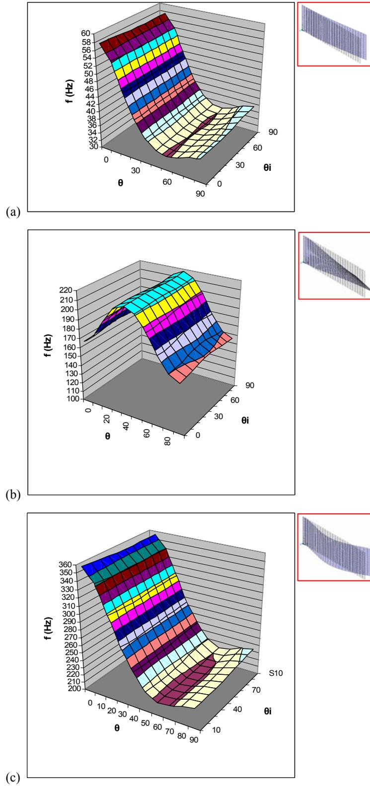
Figure 4. Resonance freq. for 3-layer board (a) 1<sup>st</sup> mode - bending, (b) 2<sup>nd</sup> mode- torsional, and (c) 3<sup>rd</sup> mode-bending
