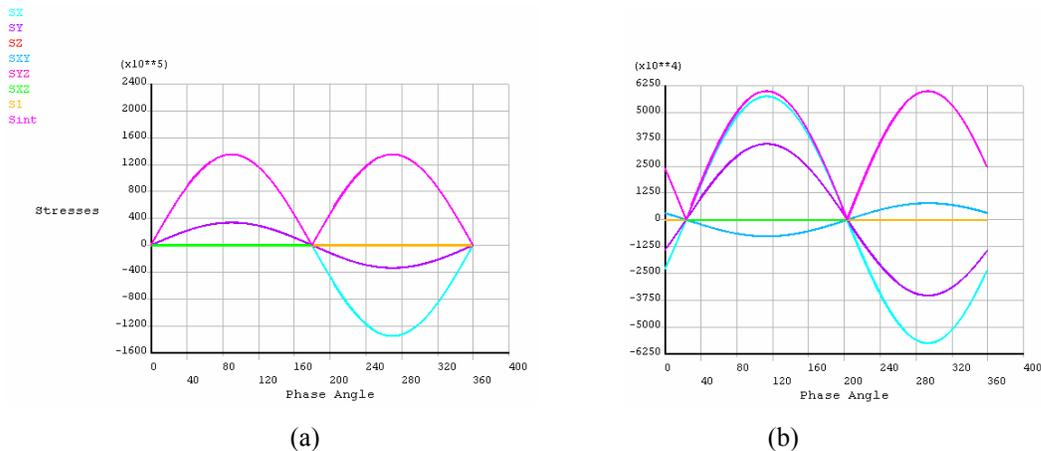
**Figure 5. Stress components vs. time (phase angle) in a cycle: (a) board with  $\theta=0^\circ$  (b) board with  $\theta=50^\circ$**
