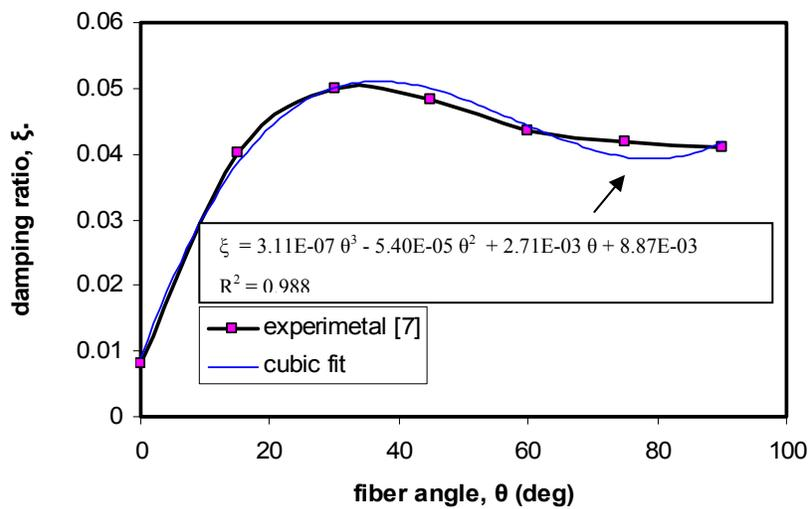
Figure 1. Typical damping ration for a glass composite
