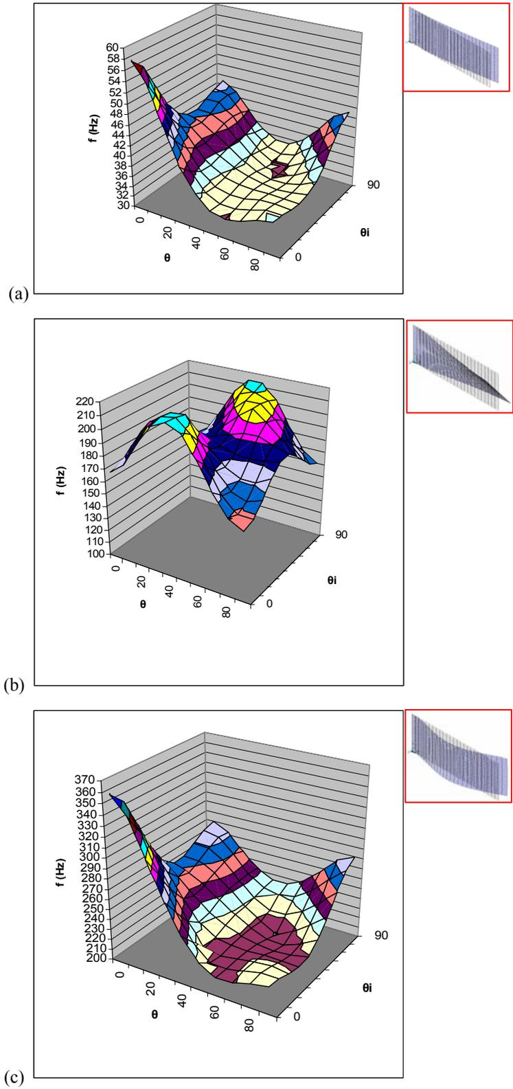
Figure 3. Resonance freq. for 2-layer board (a) 1<sup>st</sup> mode - bending, (b) 2<sup>nd</sup> mode- torsional, and (c) 3<sup>rd</sup> mode-bending
