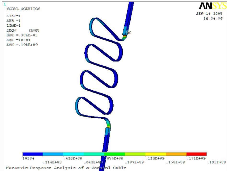
Figure 11. Von Mises stresses
