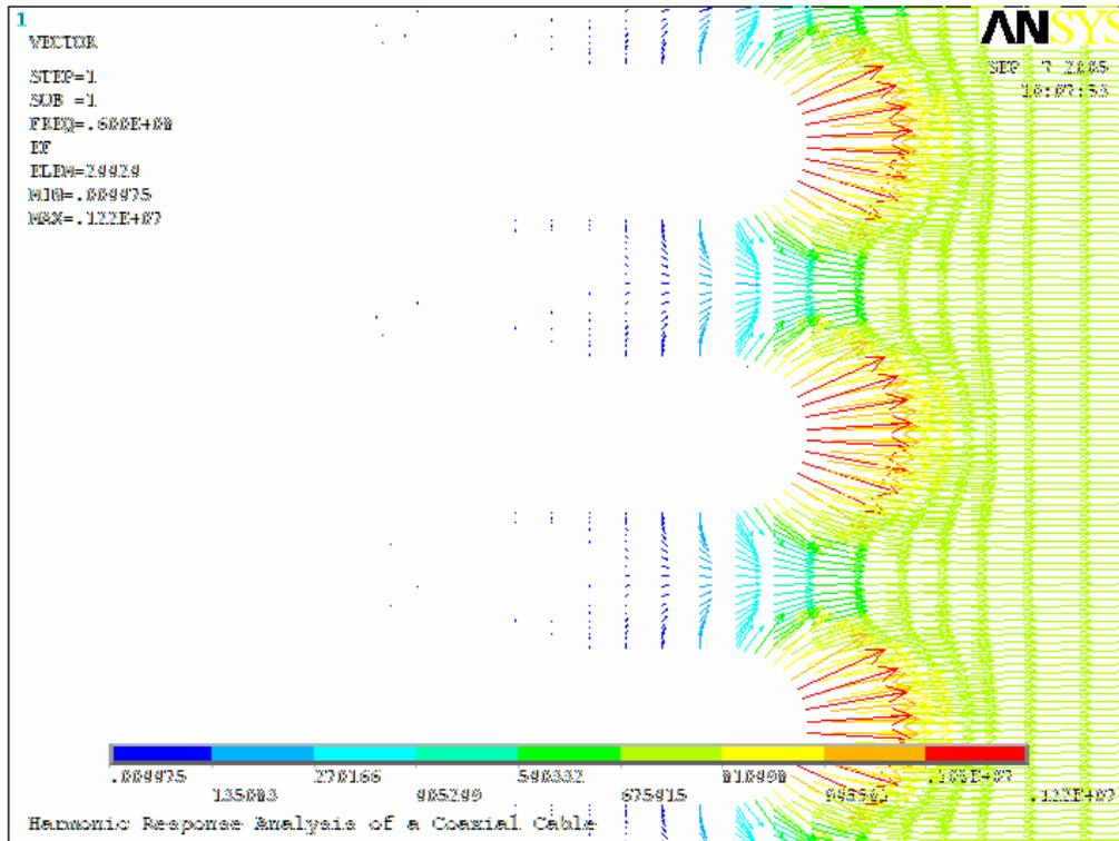
Figure 5. Electric field Real Part
