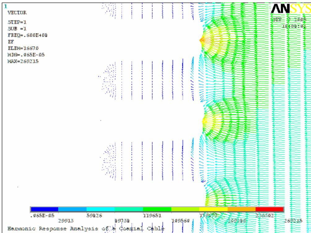
Figure 6. Electric field Imag Part
