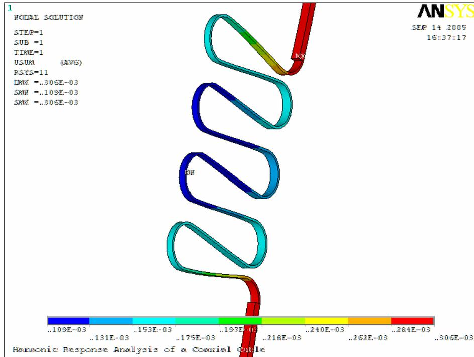
Figure 12. Displacement amplitude
