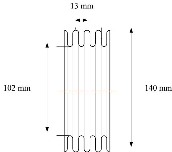
**Figure 2. Bellows geometry**
