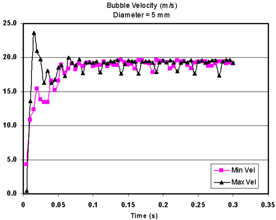
Figure 4. Bubble velocity as a function of time, 5 mm diameter
