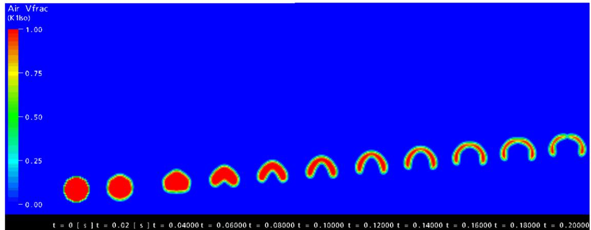
**Figure 8. The rise of the 40 mm diameter bubble**
