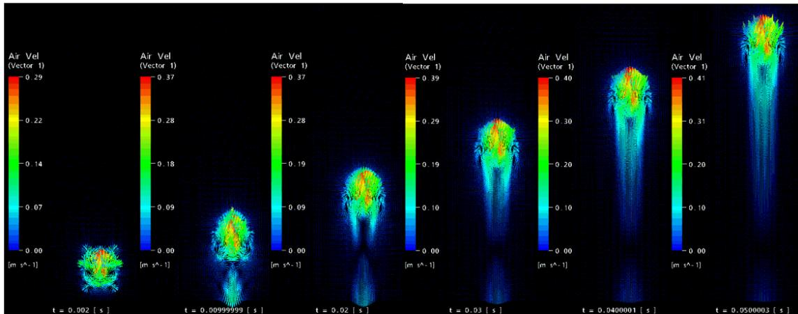
**Figure 9. Development of the velocity field for a 1 mm bubble**
