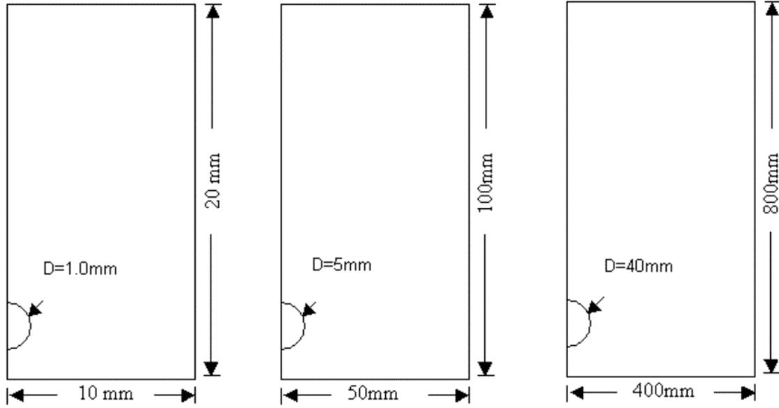
**Figure 1. Dimensions used for the CFD model**
