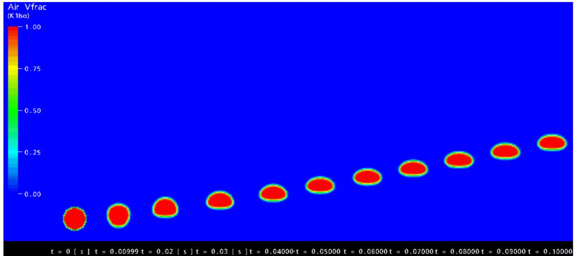
**Figure 7. The rise of the 5 mm diameter bubble**
