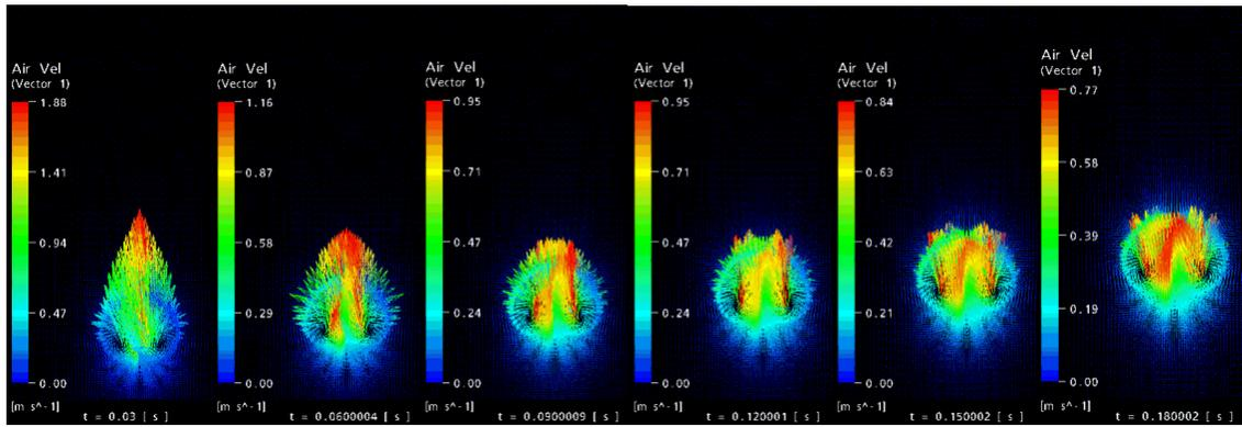
Figure 11. Development of the velocity field for a 40 mm bubble
