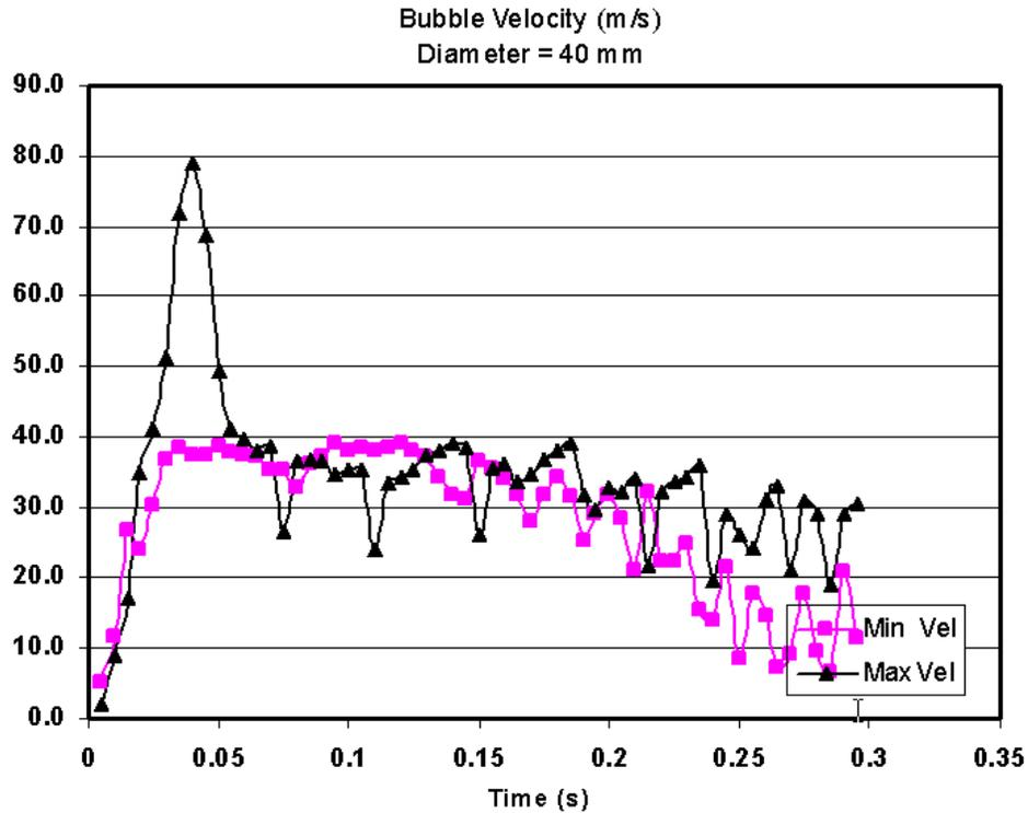
**Figure 5. Bubble velocity as a function of time, 40 mm diameter**
