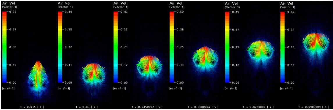
Figure 10. Development of the velocity field for a 5 mm bubble
