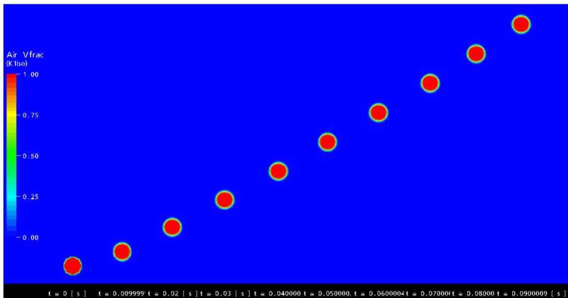
**Figure 6. The rise of the 1 mm diameter bubble**
