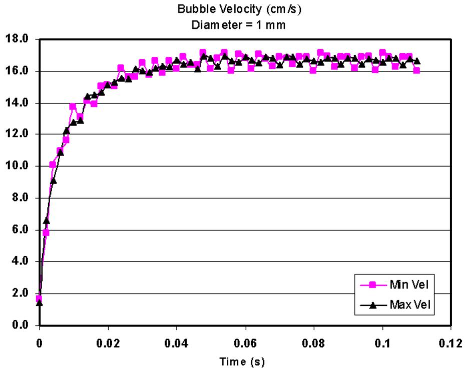
Figure 3. Bubble velocity as a function of time, 1 mm diameter
