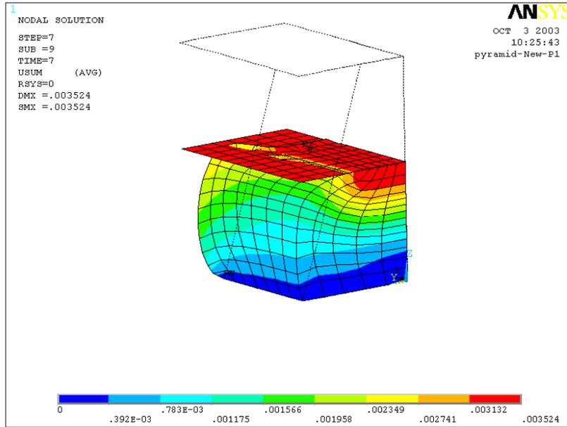
**Figure 11. Deformed shape of type 2 spacer**
