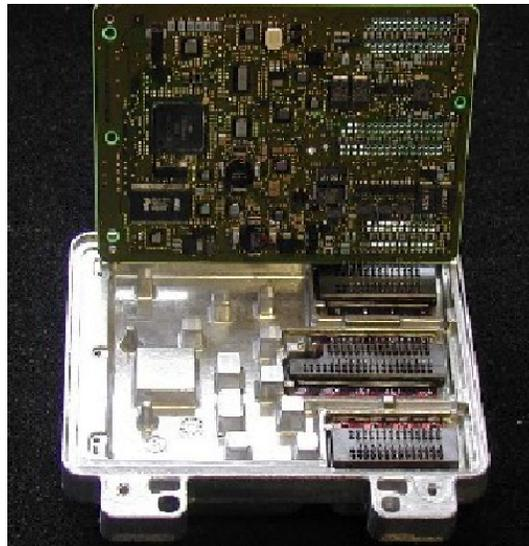
**Figure 2. Housing and circuit board assembly**
