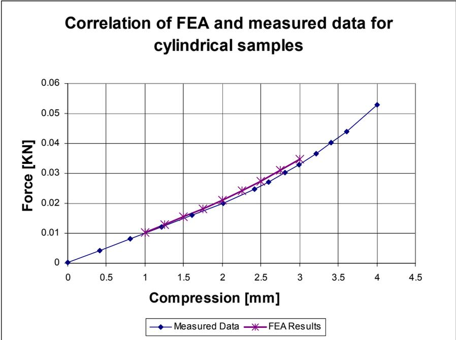
**Figure 9. Comparison of results for cylindrical samples**
