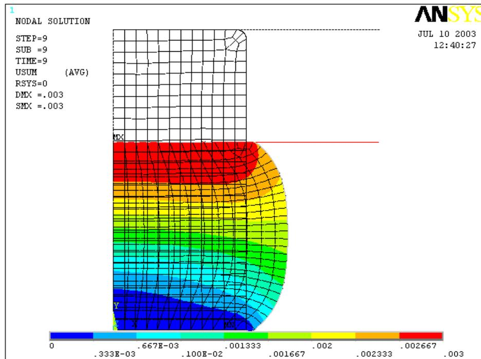
Figure 8. Deformation of the cylindrical sample
