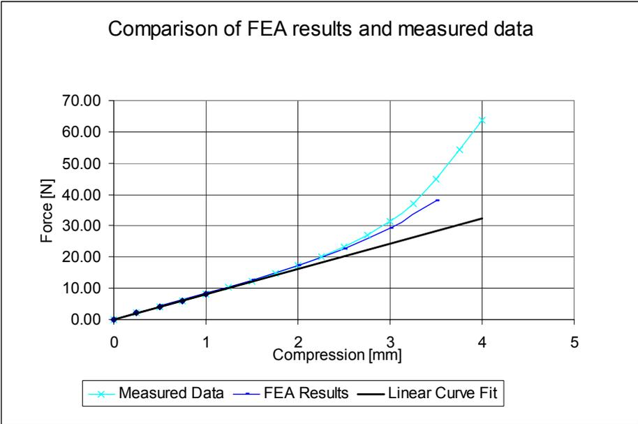
**Figure 10. Comparison of results for Type 2 spacers**
