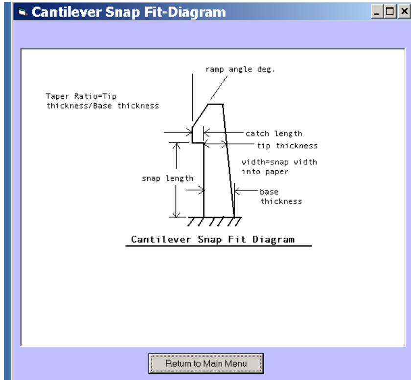
**Figure 3. Diagram of Classical Analysis Tapered Snap Fit**
