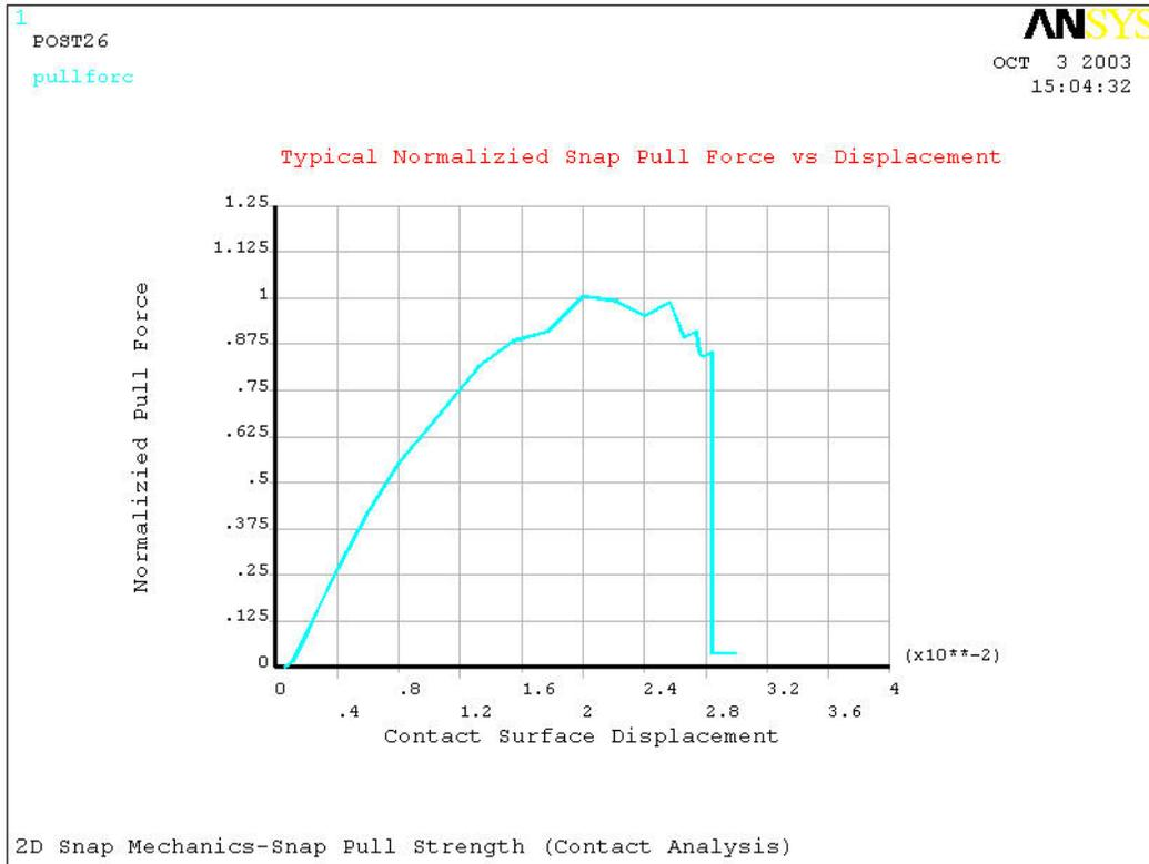
**Figure 6. Typical Normalized Snap Pull Force vs Deflection**
