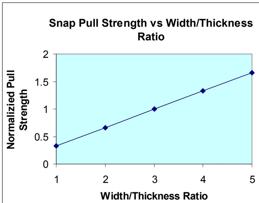
Figure 10. Snap Pull Strength vs Snap Width
