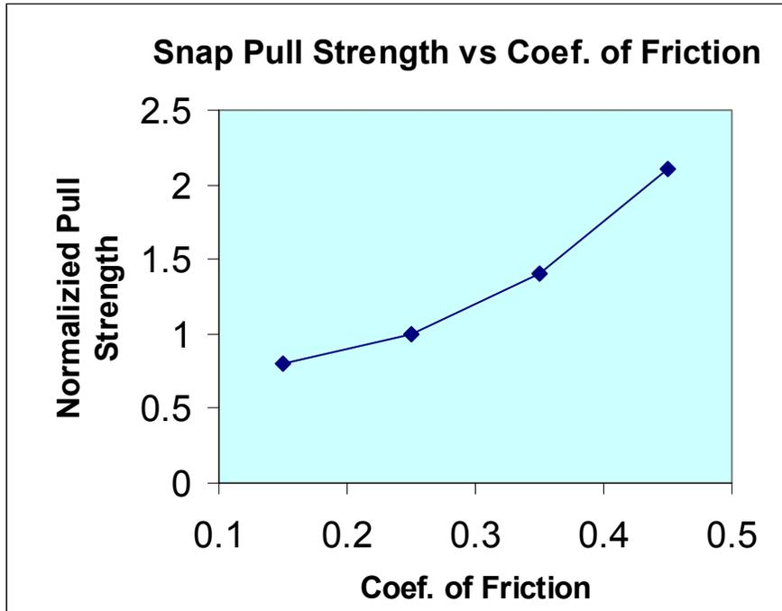
Figure 9. Snap Pull Strength vs Coef. of Friction
