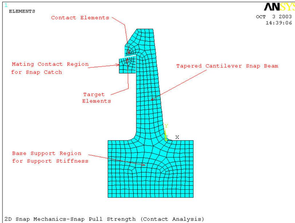
**Figure 1. Finite Element Model of Tapered Cantilever Snap Joint**
