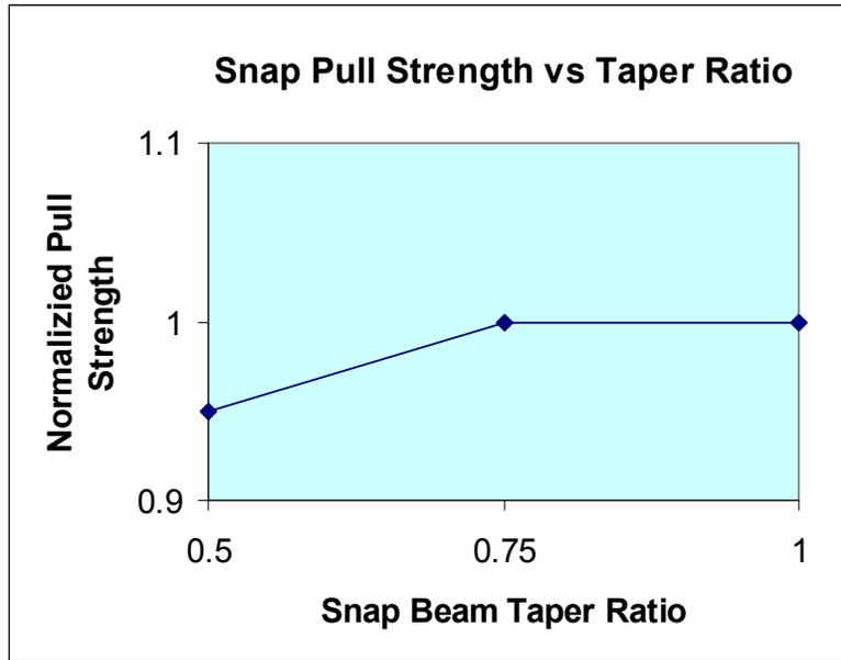
**Figure 11. Snap Pull Strength vs Snap Beam Taper Ratio**
