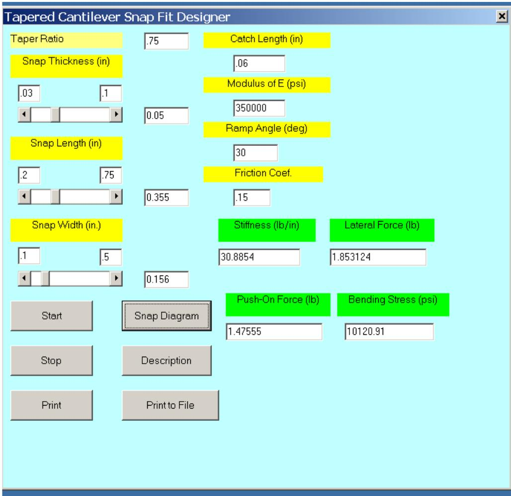
Figure 4. Tapered Beam Snap Fit Visual Basic Program
