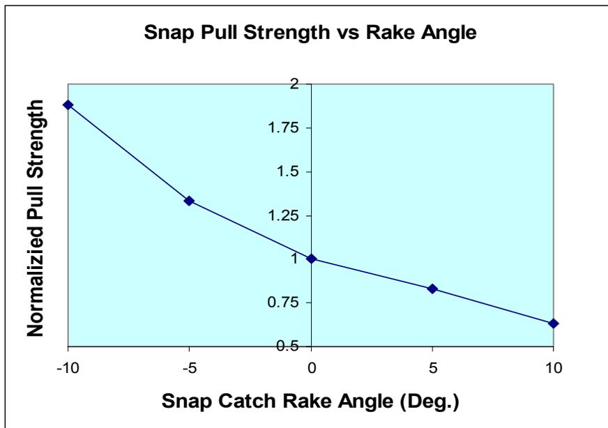
Figure 8. Snap Pull Strength vs Rake Angle
