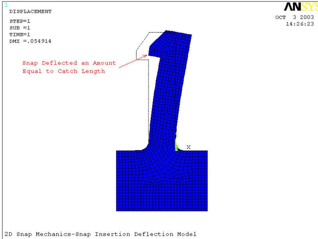
**Figure 2. Snap Fit Insertion Deflection and Stress Model**
