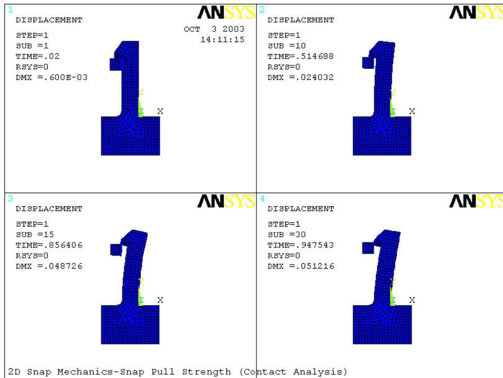
**Figure 5. Deflection Sequence of Snap Cam Out Shown In Four Frames**
