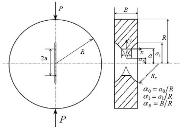
**Figure 5. The CCNBD specimen**
