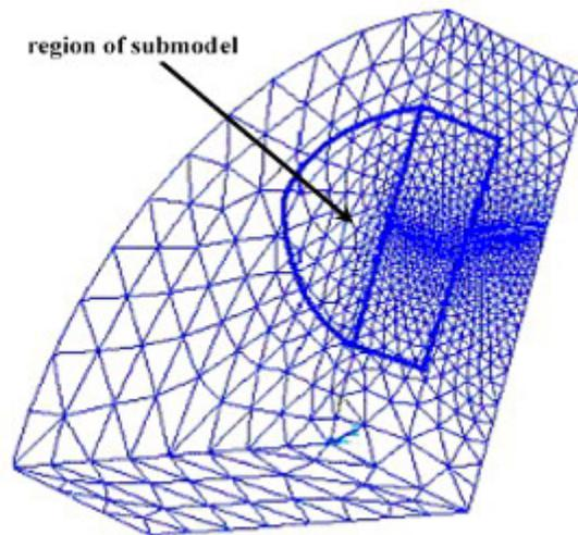
**Figure 6. The mesh of the whole Model**
