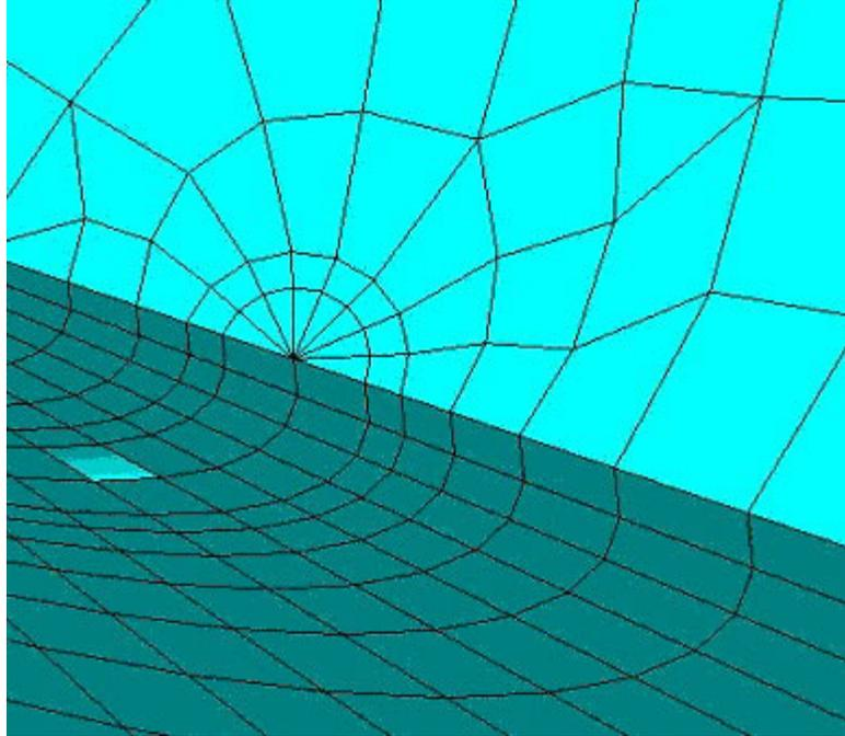
**Figure 11. Enlarged crack-tip elements**
