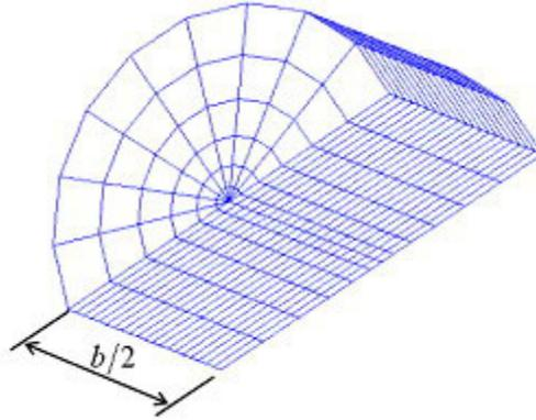
**Figure 7. The mesh of the partial crack submodel**
