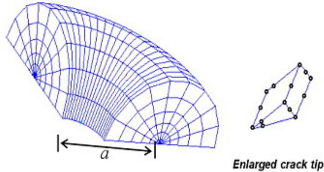
**Figure 2. The submodel of the penny-shaped crack**
