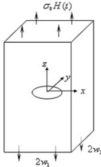
**Figure 9. Penny-shaped crack in a finite cube**
