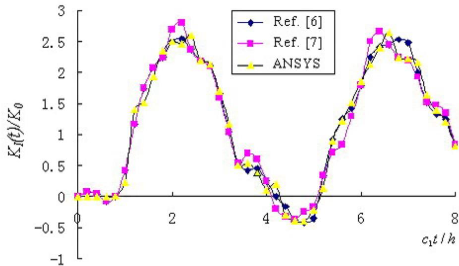
**Figure 12. Dynamic stress intensity factor of the penny-shaped crack in a finite cube**
