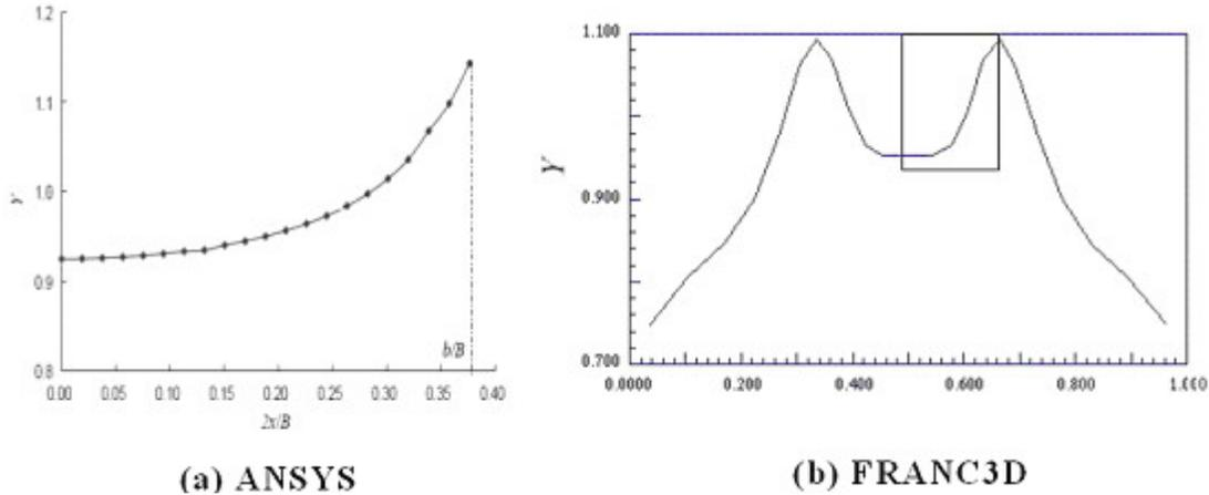
Figure 8. The distribution of the dimensionless SIF of the CCNBD specimen with  $\alpha = 0.49$
