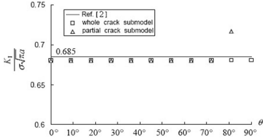
**Figure 4. The comparison of the results between the whole crack submodel and partial crack submodel**
