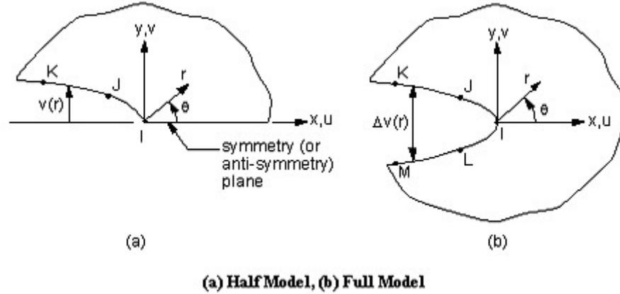
Figure 1. Nodes used for the approximate crack-tip displacements
