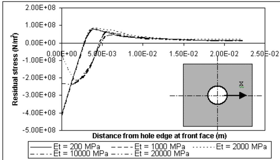
Figure 3. Variation of residual tangential stresses over the plate front face for five different material models
