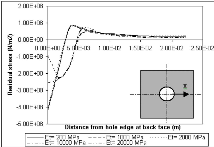
**Figure 5. Variation of residual tangential stresses over the plate back face for five different material models**
