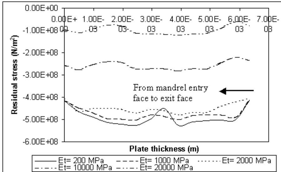
**Figure 6. Variation of residual stresses through the plate thickness for five different material models**
