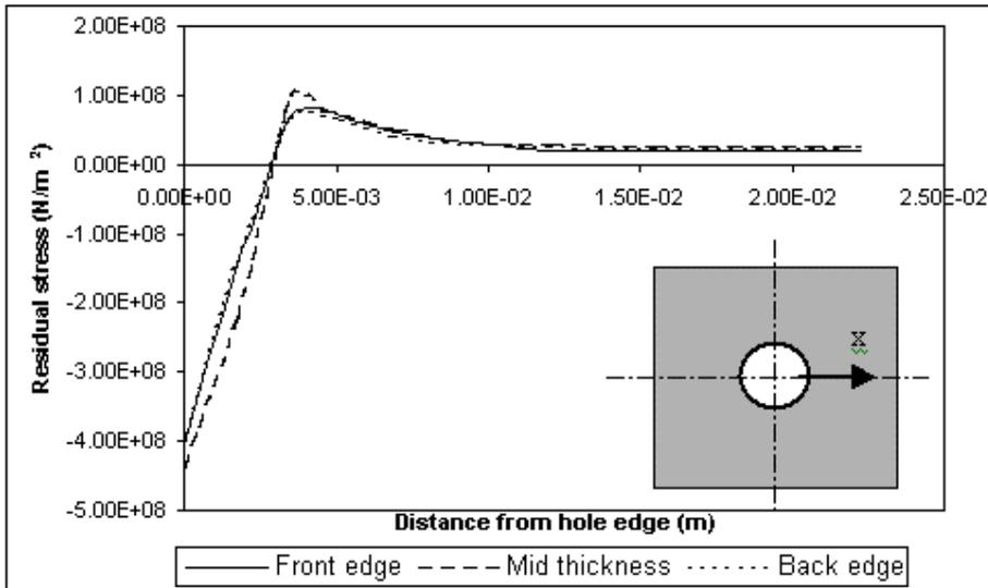
Figure 2. Variation of residual tangential stresses along the plate edges ( $E_t = 200 \text{ MPa}$ )
