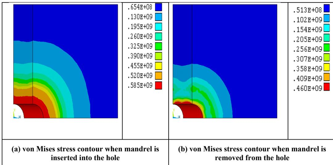
**Figure 1. von Mises stress contours due to cold expansion ( $E_t = 200 \text{ MPa}$ )**
