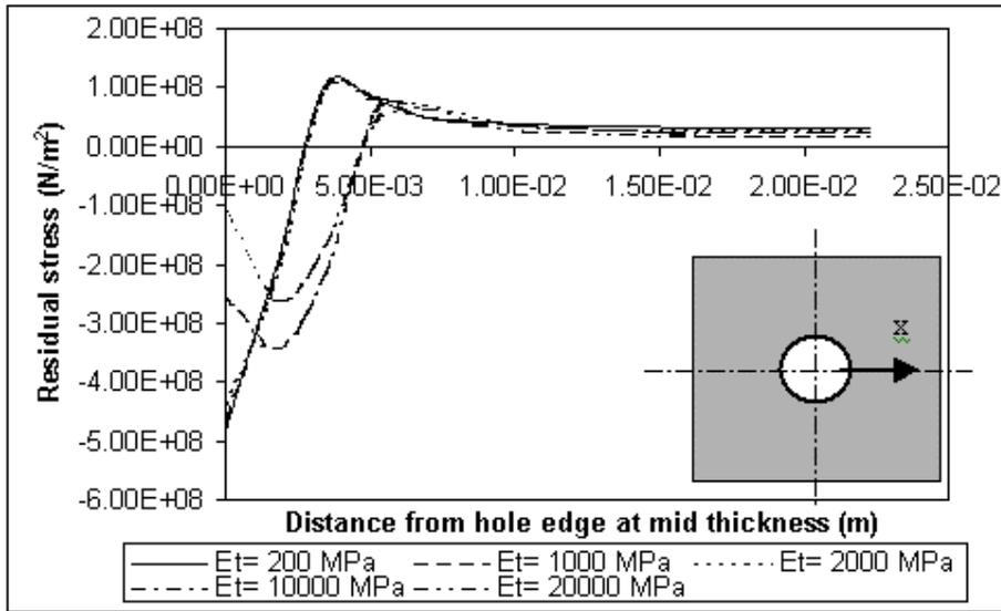
**Figure 4. Variation of residual tangential stresses along the plate mid thickness for five different material models**
