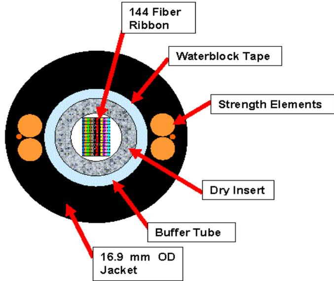
Figure 4. Test 1 Cable Design
