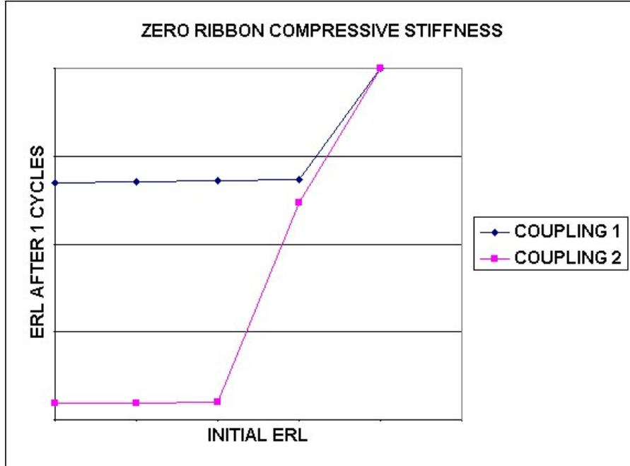
Figure 8. Maximum ERL after Loading Versus Initial ERL, Zero Ribbon Compressive Stiffness
