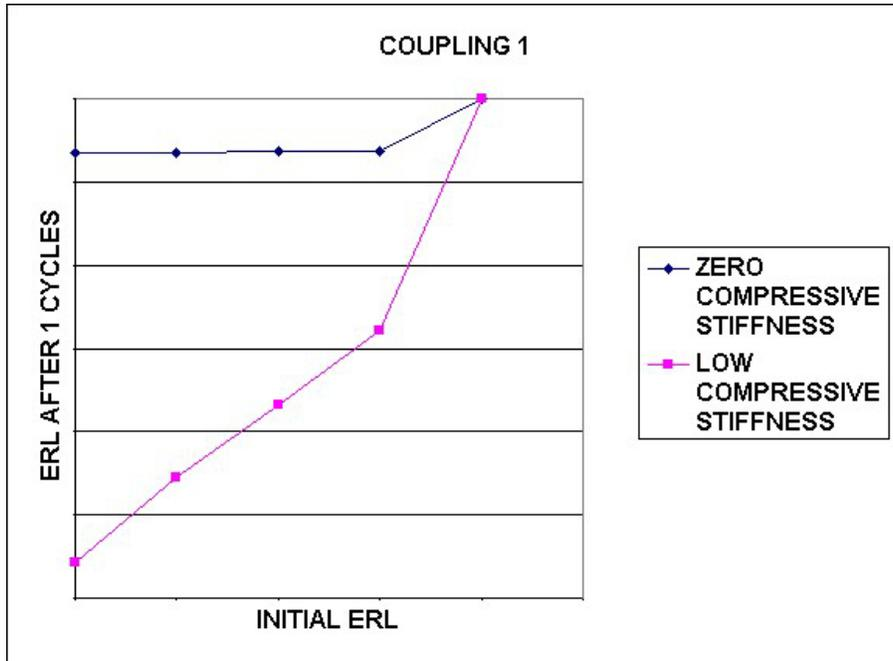
**Figure 10. Maximum ERL after Loading Versus Initial ERL, Low Ribbon/Jacket Coupling**
