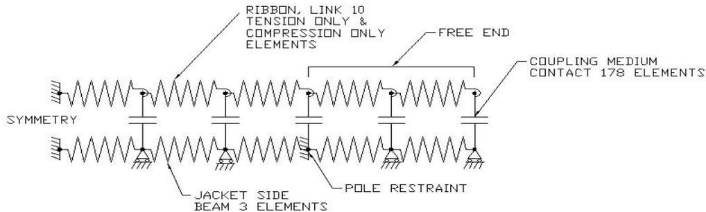
**Figure 3. Aerial Cable Finite Element Model Schematic**
