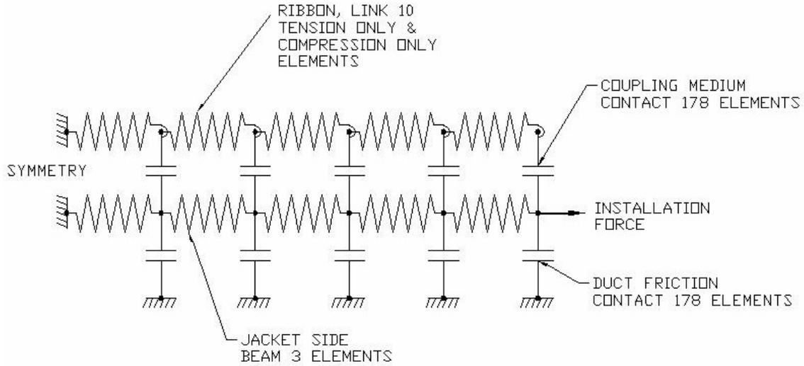
**Figure 2. Duct Installation Finite Element Model Schematic**
