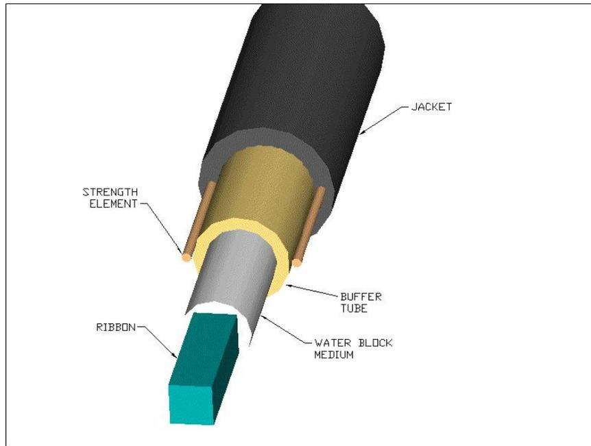
**Figure 1. Dry Single Tube Cable Construction**
