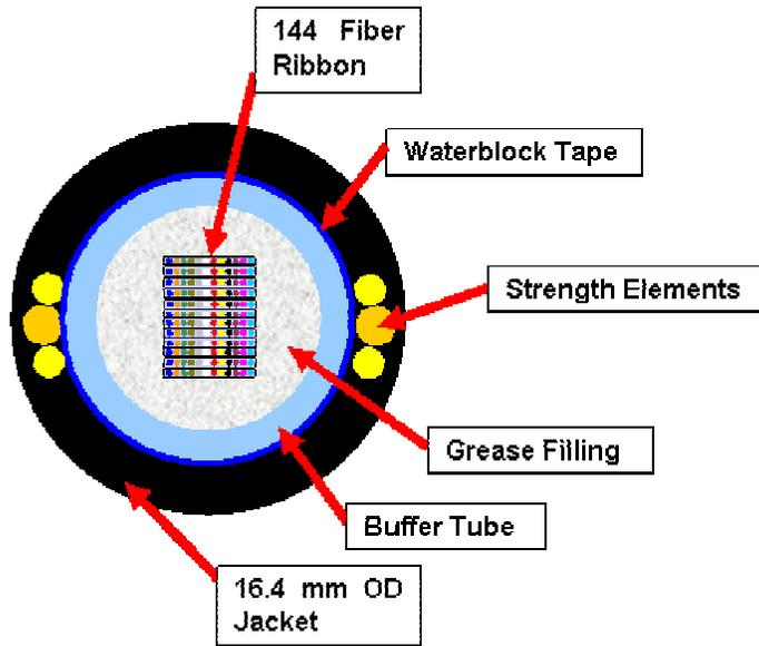
Figure 5. Test 2 Cable Design
