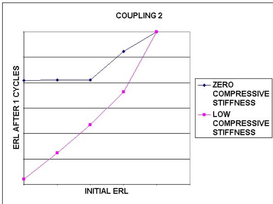
**Figure 11. Maximum ERL after Loading versus Initial ERL, High Ribbon/Jacket Coupling**
