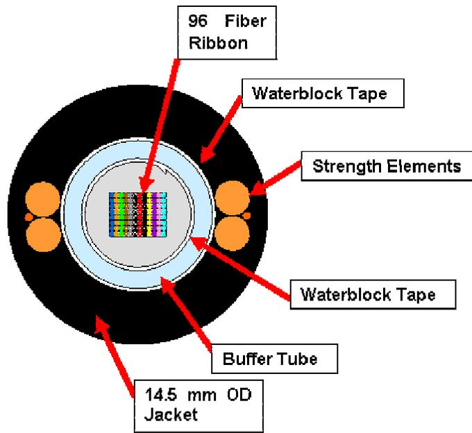
Figure 6. Test 3 Cable Design
