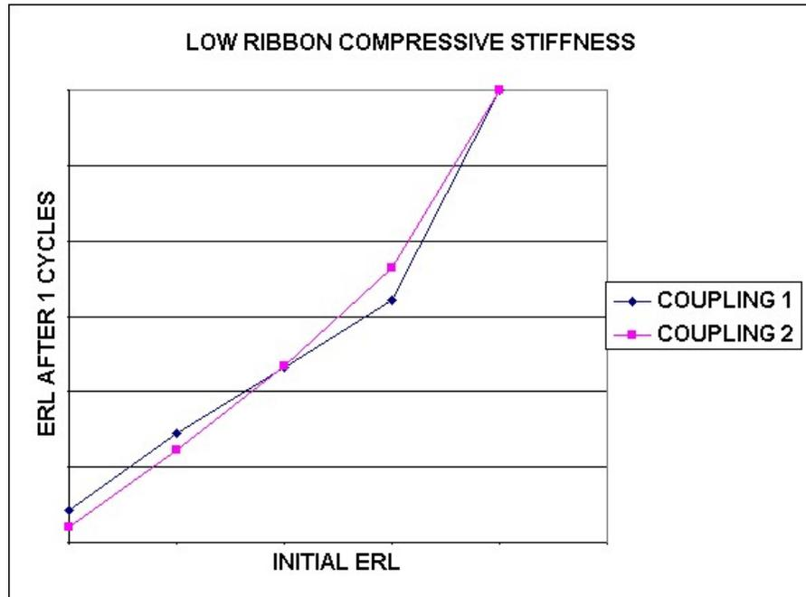
Figure 9. Maximum ERL after Loading Versus Initial ERL, Low Ribbon Compressive Stiffness
