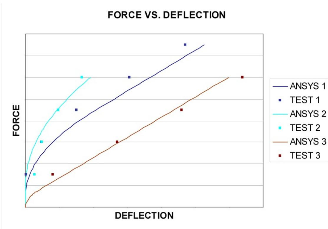
Figure 7. ANSYS Results Comparison with Test
