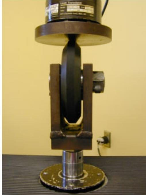
**Figure 5. Front View - Radial Load Versus Deflection for Neoprene Stiffness**
