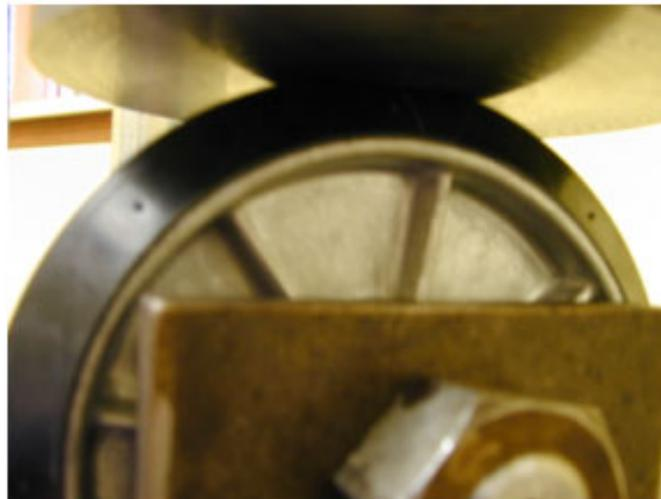
**Figure 6. Side View - Radial Load Versus Deflection for Neoprene Stiffness**
