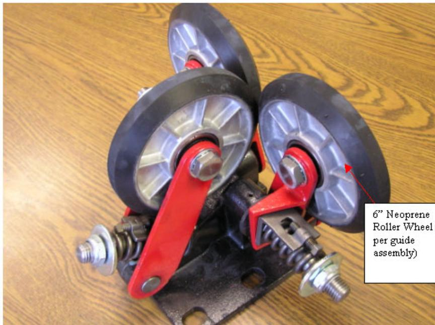
**Figure 1. Moderate Speed Roller Guide**
