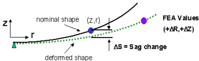
Figure 8. Radial Correction
