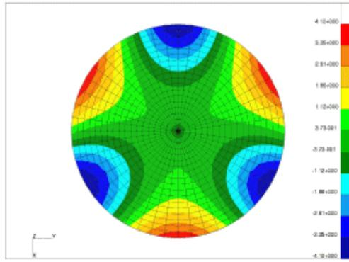
**BFP and Power Removed in SigFit RMS=1.6 $\lambda$**
