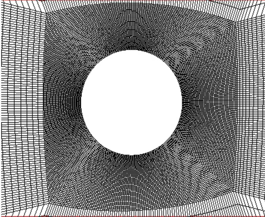
**Figure 6. Final Grid at Tube**
