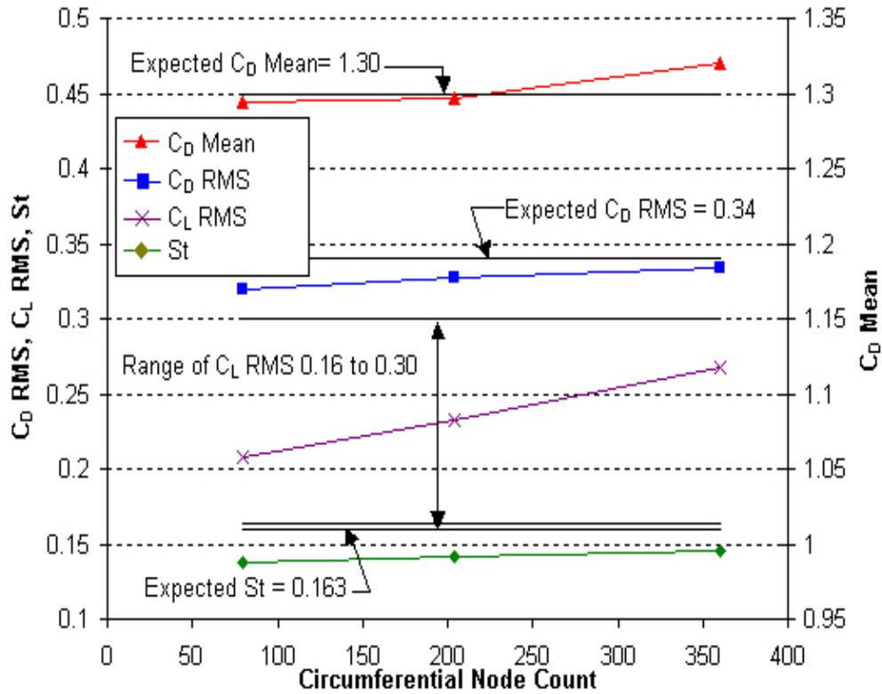
**Figure 5. Circumferential Node Number Dependence of Solution ( $Re = 100$ , Timestep = 0.005 seconds)**
