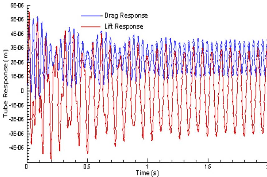
**Figure 9. Tube Response: Reynolds No = 1000 (dt = 0.002, Grid Res: 360 circ. nodes)**
