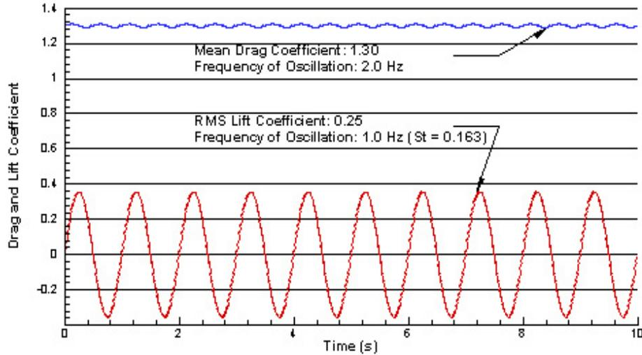
Figure 3. Expected Lift/Drag Coefficient History, Re = 100
