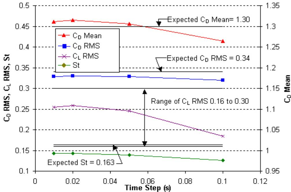
Figure 7. Time Step Dependence ( $Re = 100$ , Grid Res: 204 circ. nodes)
