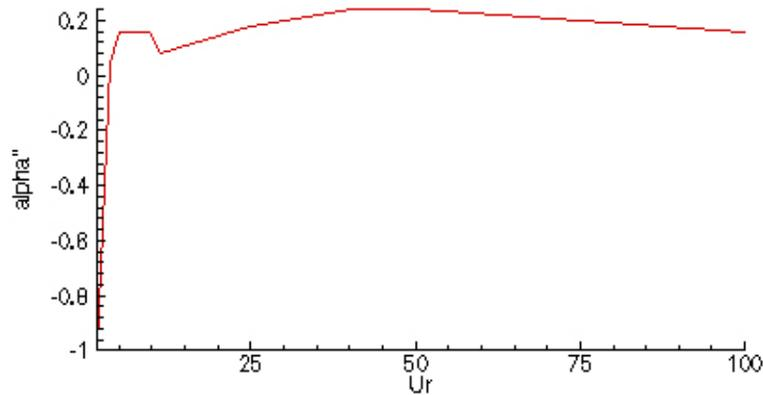
**Figure 1. Experimental Fluid Force Coefficient  $\bar{\alpha}'_{11}$**
