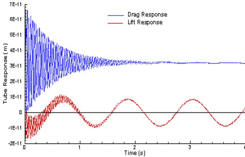
**Figure 8. Tube Response: Reynolds No = 100 (dt = 0.02, Grid Res: 360 circ. nodes)**
