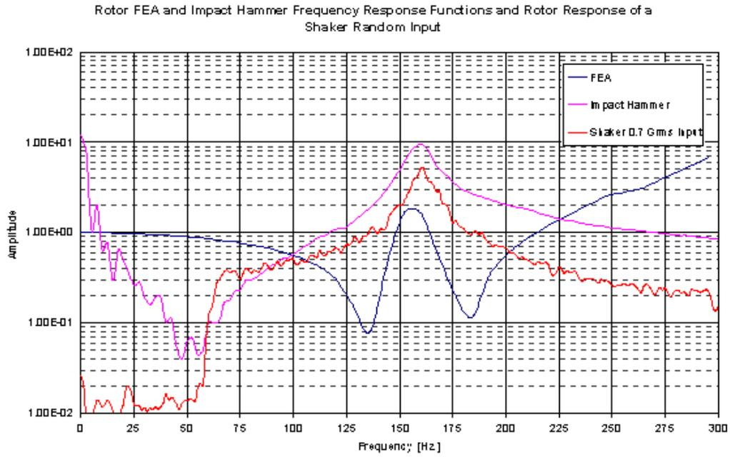
**Figure 6 - 0.7 Grms Random Input Generator Vibration Response vs. Analytical and Experimental Generator FRF**
