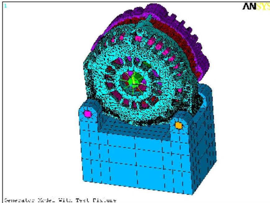
**Figure 1 - Generator Finite Element Model**
