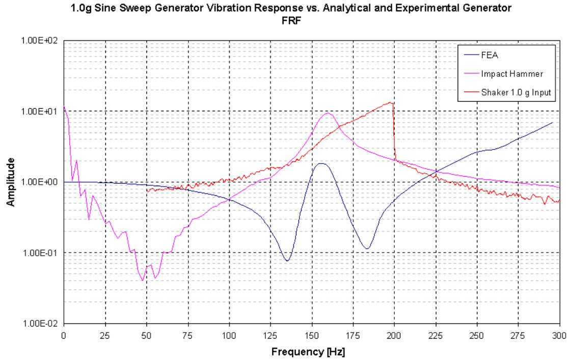
**Figure 5 - 1.0 g Sine Sweep Generator Vibration Response vs. Analytical and Experimental Generator FRF**
