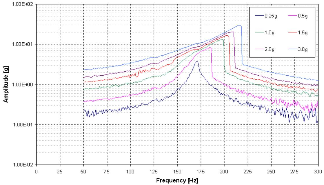
Figure 14 - Ascending Sine Sweeps – Generator Vibration Response
