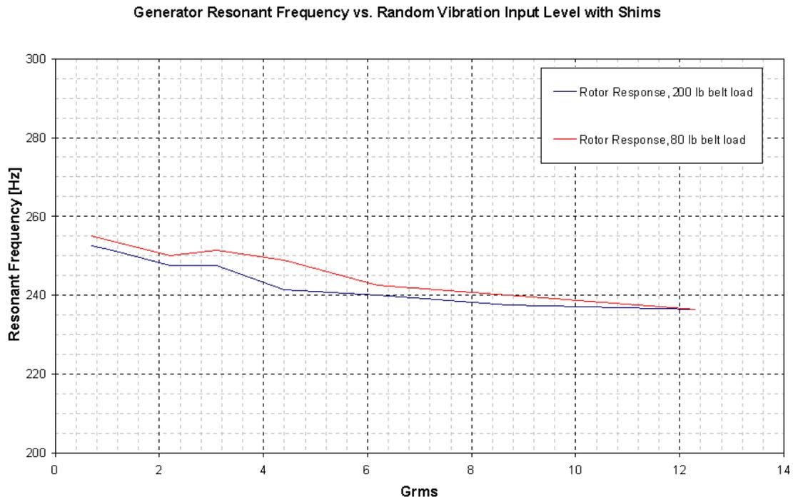
**Figure 8 - Generator Resonant Frequency vs. Random Vibration Input Level with Shims**
