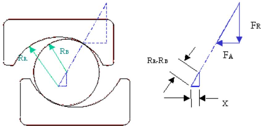
**Figure 10 - View of Axially Displaced Bearing Section**
