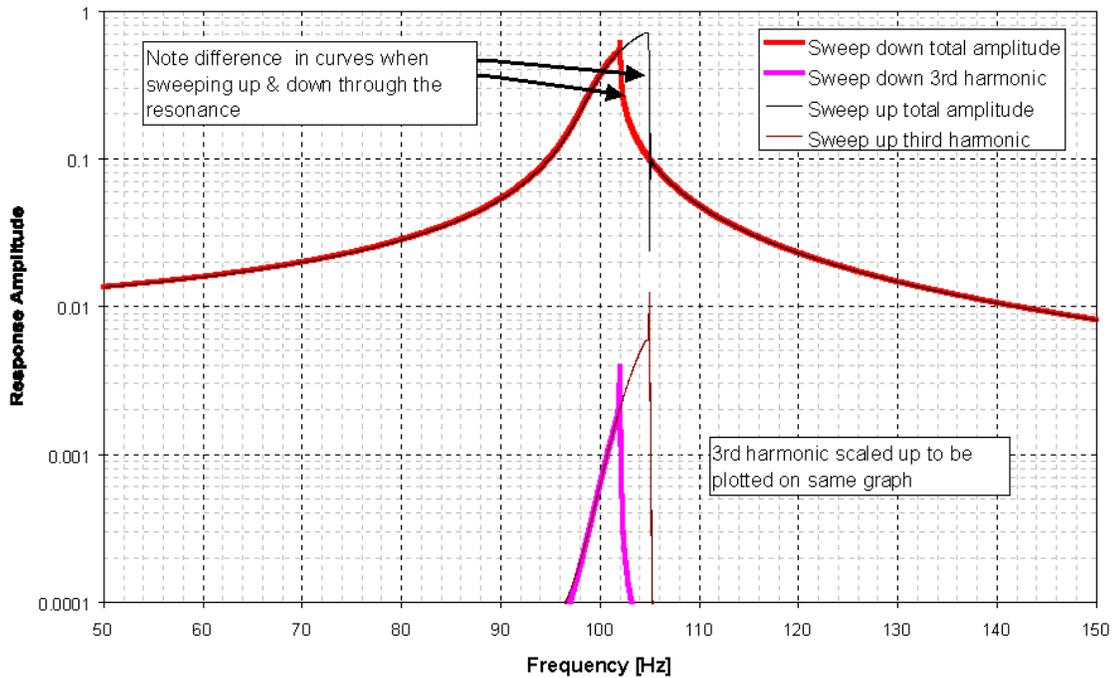
Figure 11 - Non-Linear Response - Sine Sweep Up & Down
