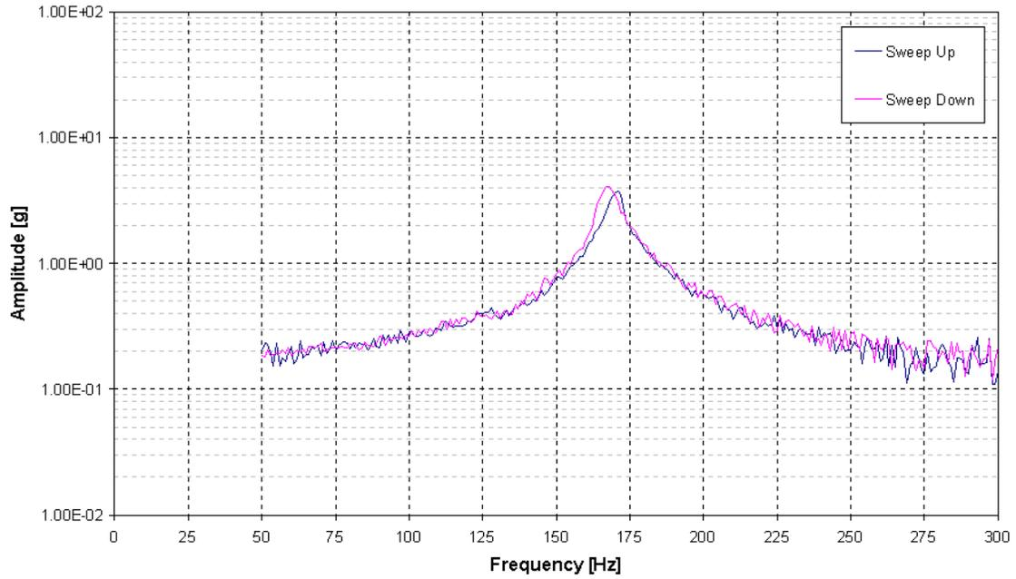
Figure 12 - 0.25 g Sine Sweep - Generator Vibration Response
