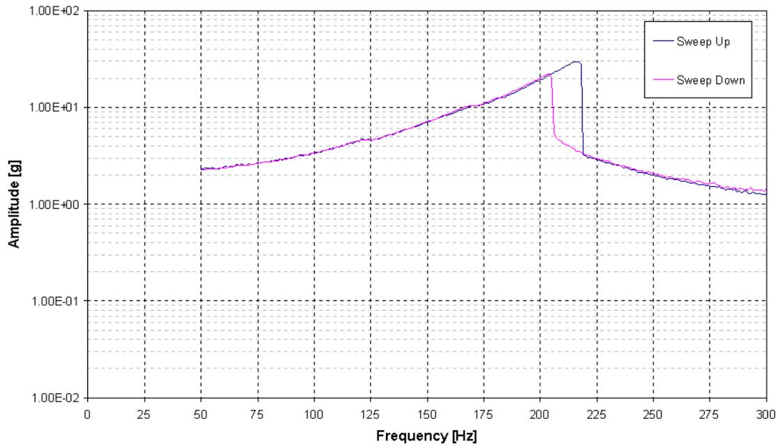
Figure 13 - 3.0 g Sine Sweep - Generator Vibration Response
