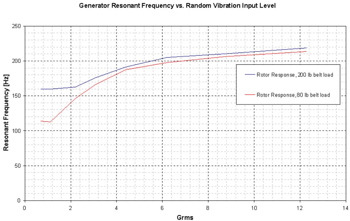
**Figure 7 - Generator Resonant Frequency vs. Random Vibration Input Level**
