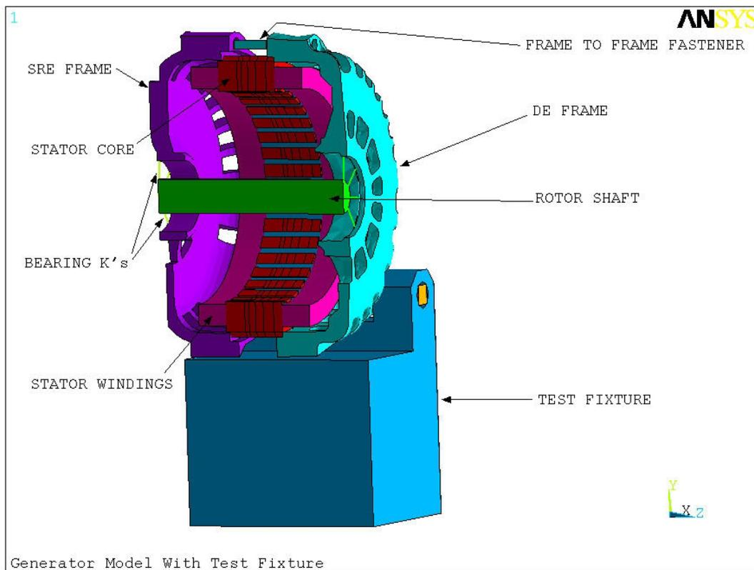
**Figure 2 - Generator Cross Section**
