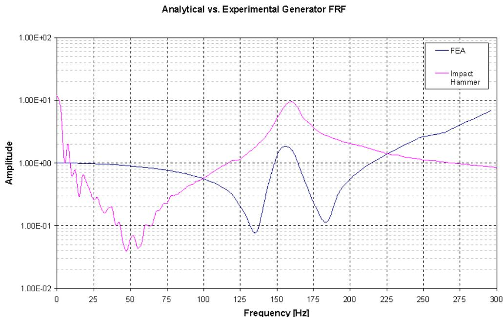
**Figure 3 - Analytical vs. Experimental Generator FRF**
