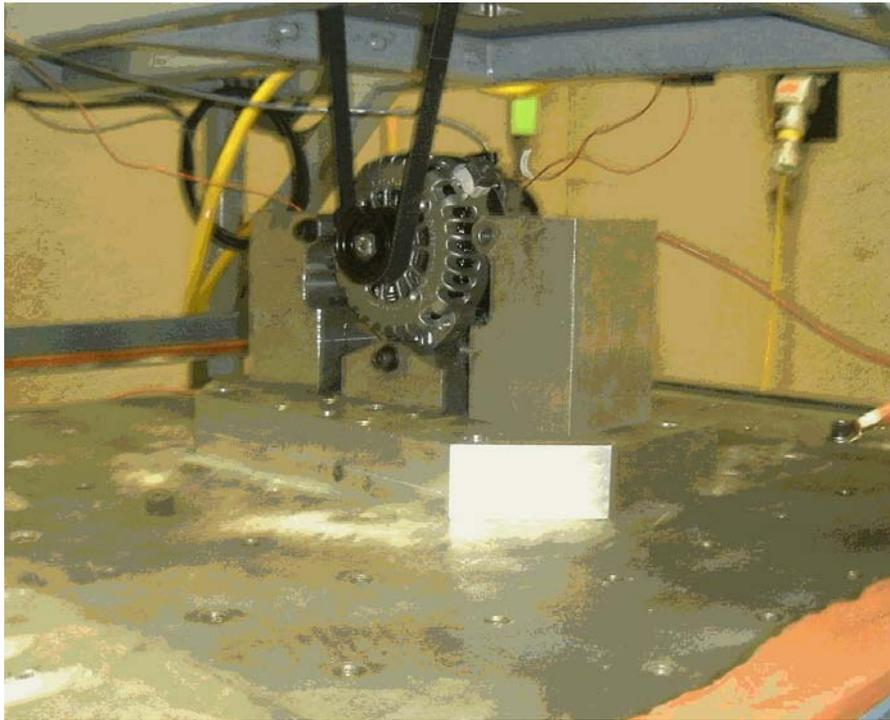
**Figure 4 - Electrodynamic Shaker Generator Test Setup**
