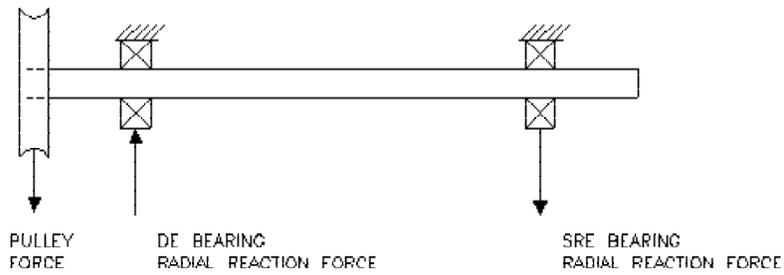
SHAFT WITH PULLEY AND TWO BALL BEARINGS
