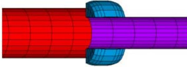
**Figure 3 - Meshed RT2 Retainer with Sections of RT1 and RT2 Solid Contacts**
