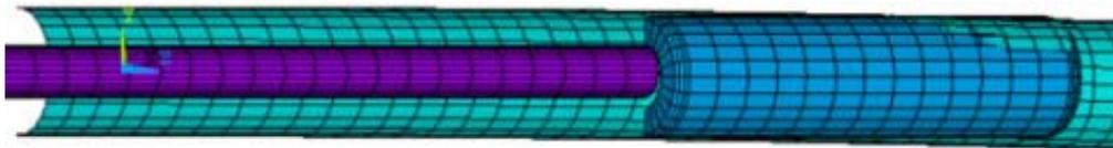
**Figure 4 - Initial Contact between Locking Tool and PT**
