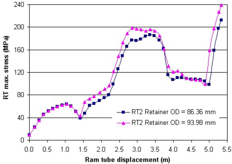
Figure 10 - RT Maximum Stress during Inspection
