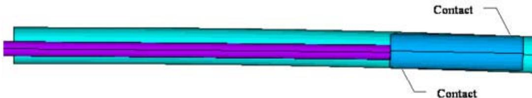
**Figure 5 - Inspection First Stage: Locking Tool Twisted Down**
