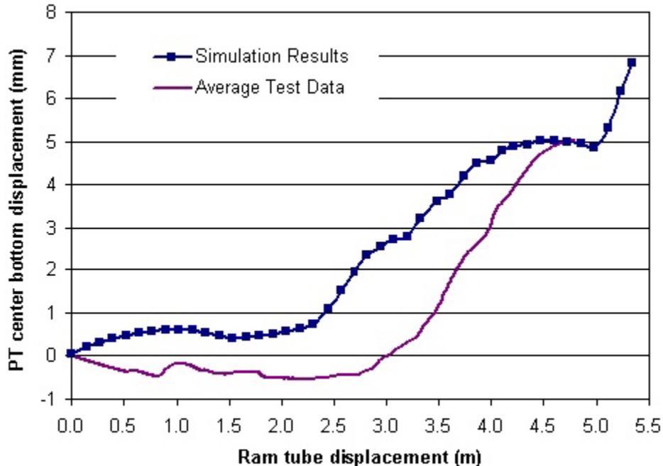
Figure 12 - Comparison with Test Data: PT Vertical Displacement
