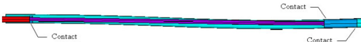
**Figure 7 - Inspection Third Stage: Locking Tool Twisted Up**
