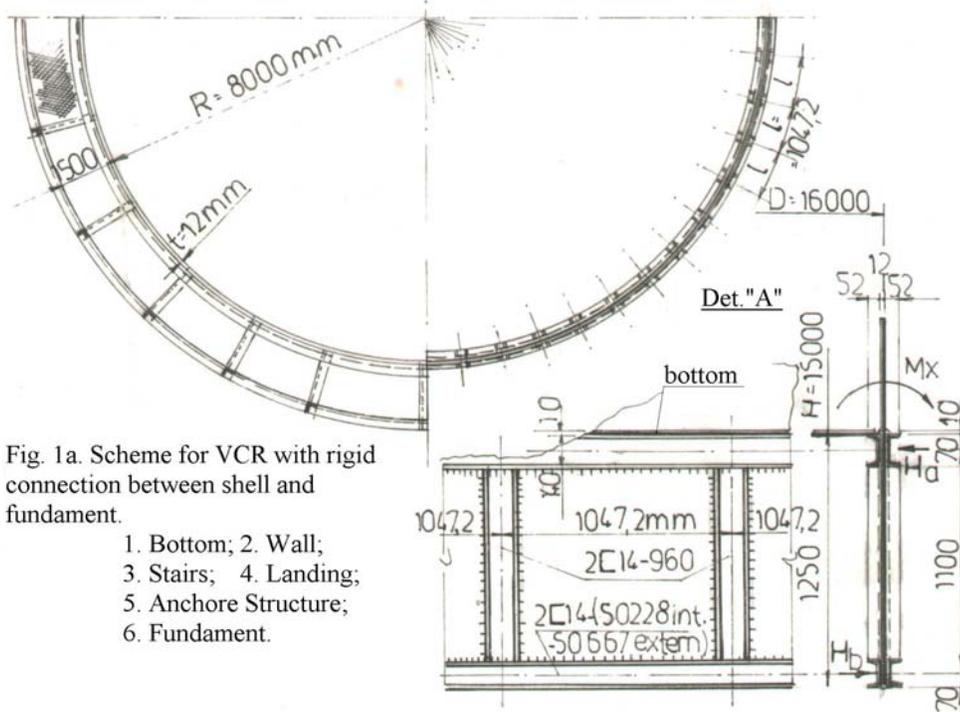
Fig. 1a. Scheme for VCR with rigid connection between shell and fundament.
