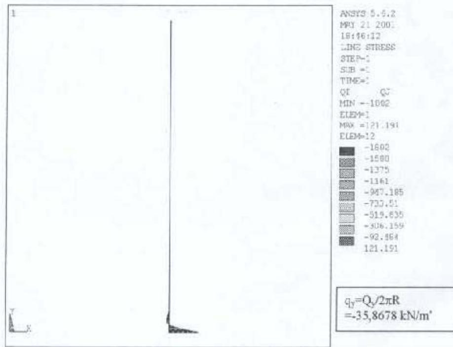
**Figure 5 - Transversal Force  $Q_x$ - diagram**
