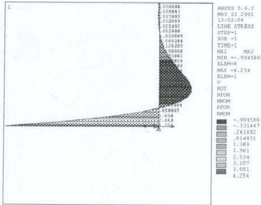
Figure 3 - Bending Moment  $M_x$ - diagram
