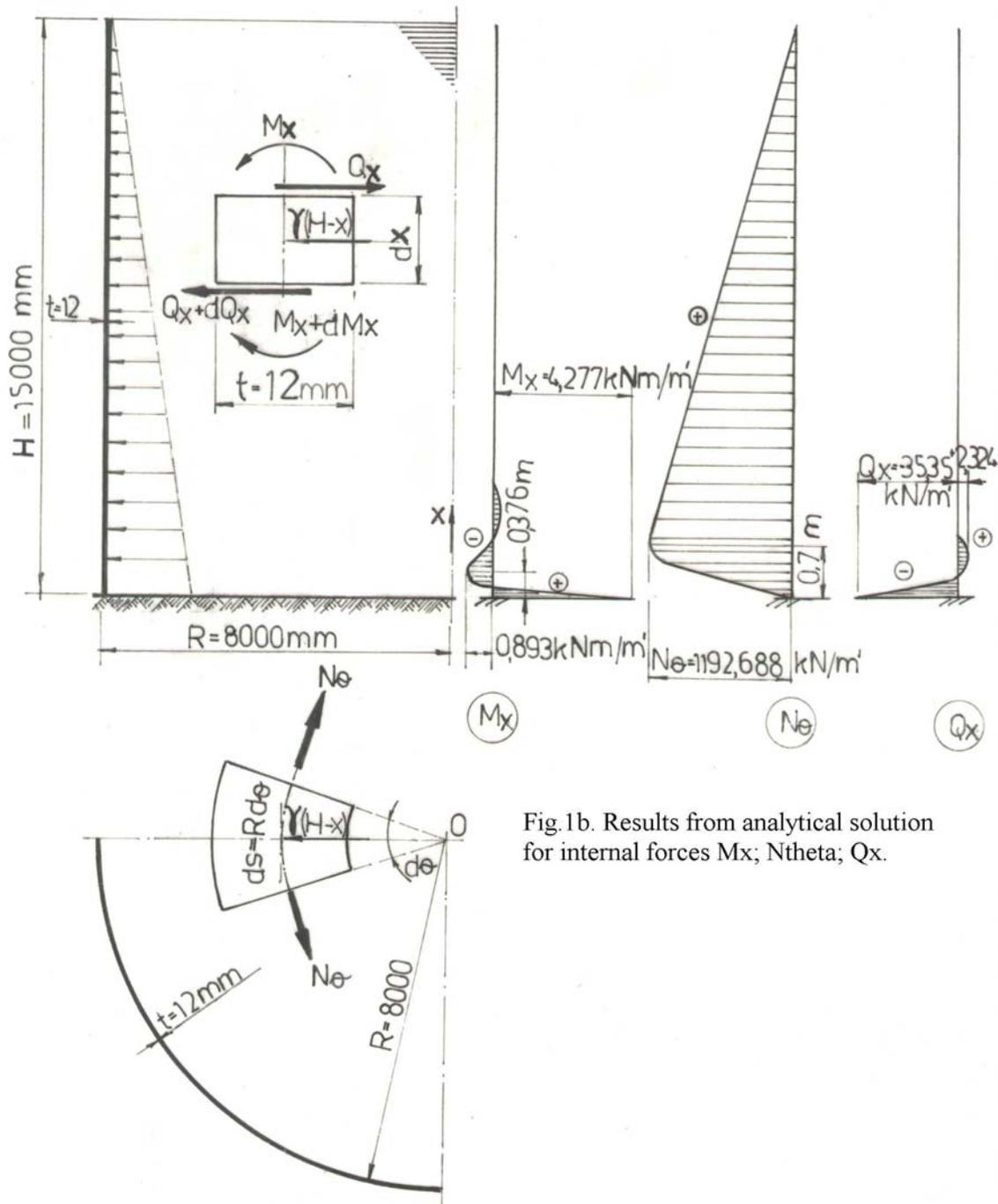
Fig.1b. Results from analytical solution for internal forces  $M_x$ ;  $N_\theta$ ;  $Q_x$ .
