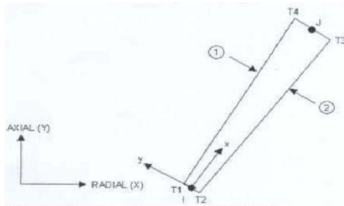
Figure 2 - Axis-symmetrical Shell element-SHELL 61
