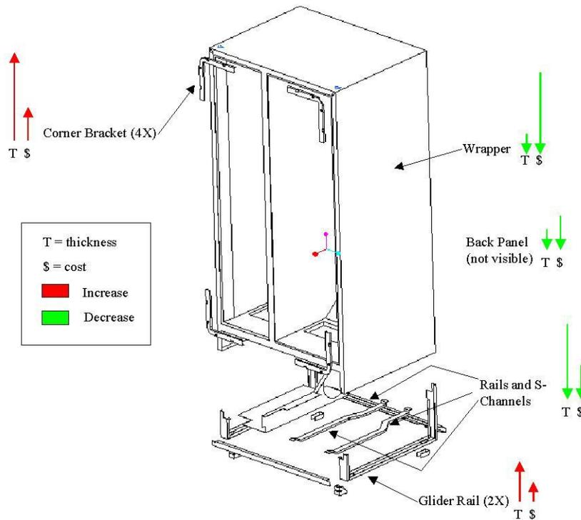
Figure 8 - Thickness and Cost Changes of Optimized Cabinet
