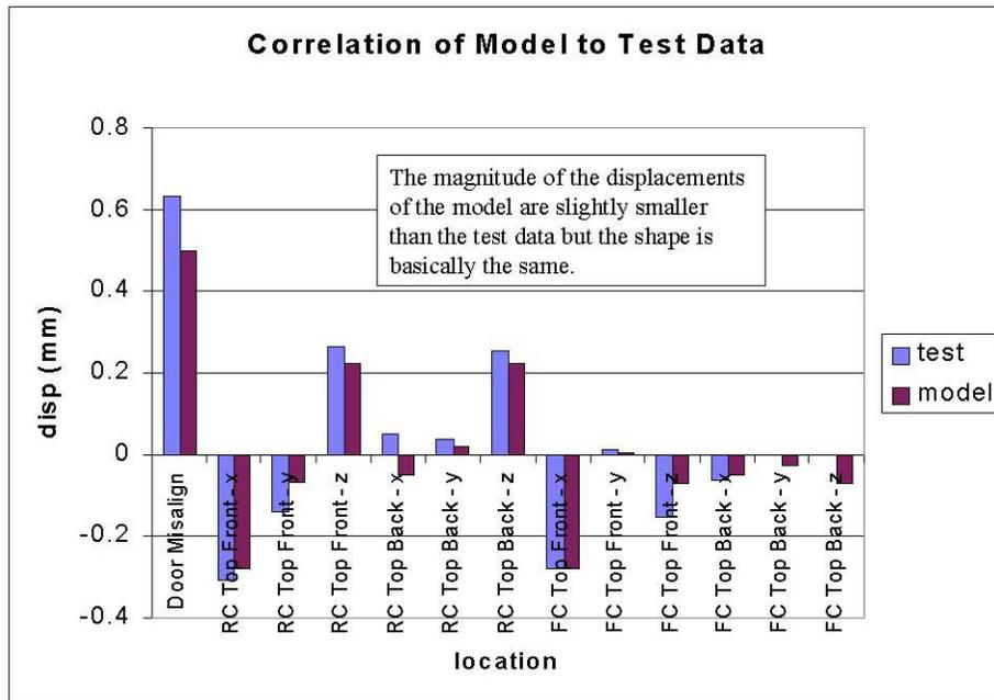
**Figure 4 - Graph Showing Correlation of Model to Test**
