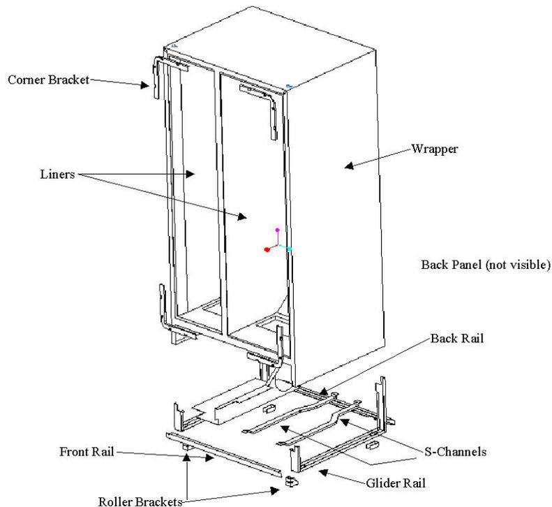
Figure 1 - Exploded View of Pro/Engineer Cabinet Model
