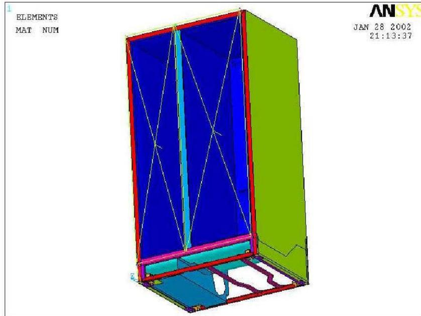
**Figure 2 - Isometric View of Ansys FE Cabinet Model**
