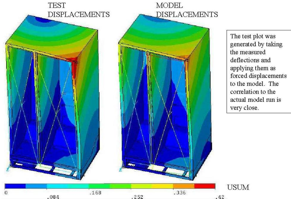
**Figure 5 - Plot Showing Correlation of Model to Test**
