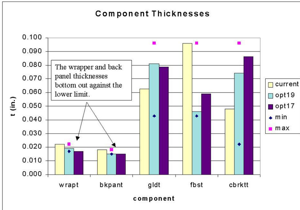
Figure 6 - Graph of Current and Optimized Thicknesses
