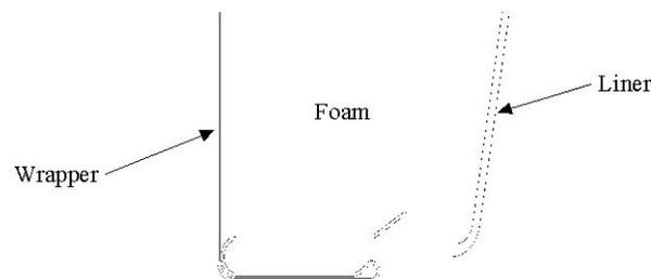
**Figure 3 - Detail of Wrapper Front Flange and Liner Flange**
