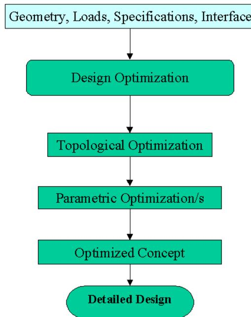
**Figure 1 - Typical Design Optimization Methodology Flowchart**
