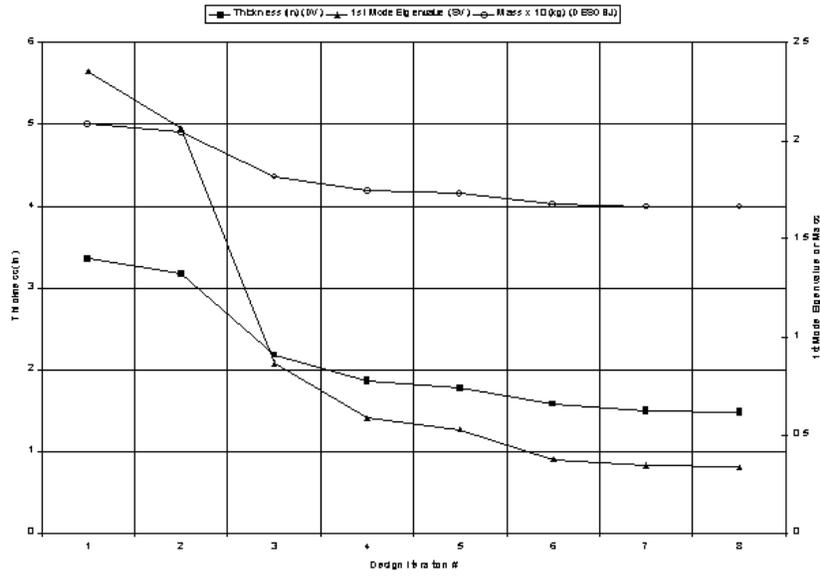
Figure 9 - Thickness Optimization Iteration History
