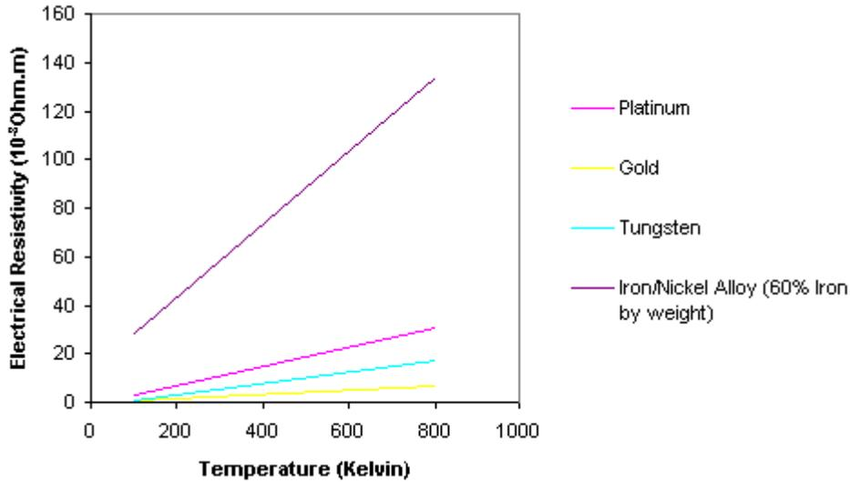
Figure 11 - Electric Properties Of Other Possible Support Arm Materials
