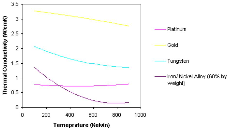
Figure 12 - Thermal Properties Of Other Possible Support Arm Materials
