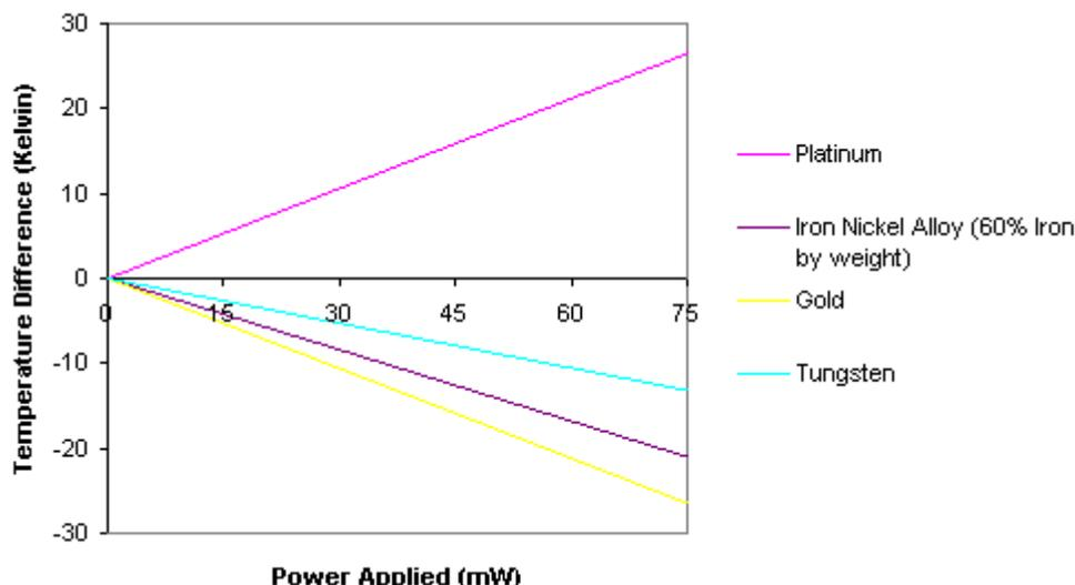
**Figure 13 - Comparison Between The Operating Temperature For A Range Of Materials**
