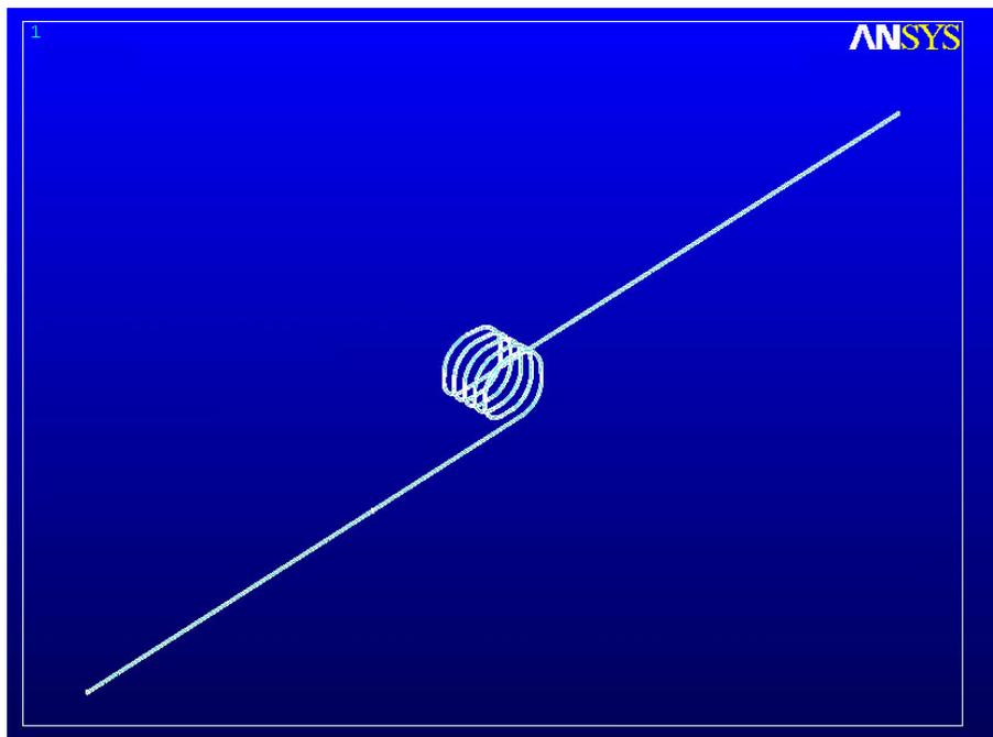
**Figure 4 - The Platinum Heating Coil**
