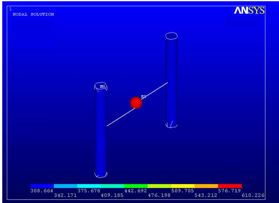
**Figure 10 - The Thermal Profile Of A Pellistor Generated Using An Input Power Of 70mw (Temperatures Are In Kelvin)**
