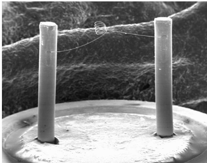
Figure 1 - Scanning Electron Microscope Photograph Of The Platinum Wire Coil Suspended Between Two Support Arms
