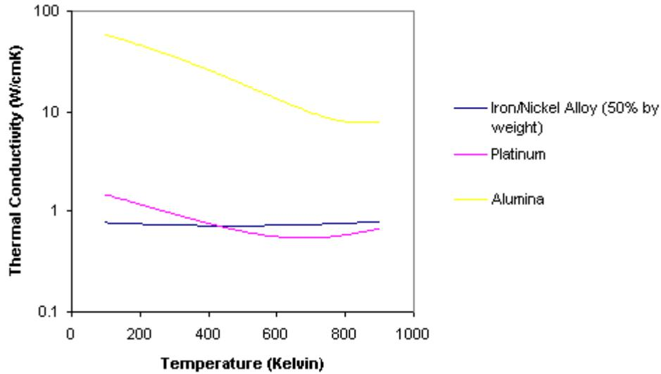
**Figure 8 - Thermal Properties Of The Materials Used To Construct Commercial Pellistors**
