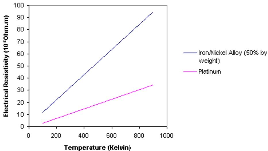
Figure 7 - Electrical Properties Of The Materials Used To Construct Commercial Pellistors
