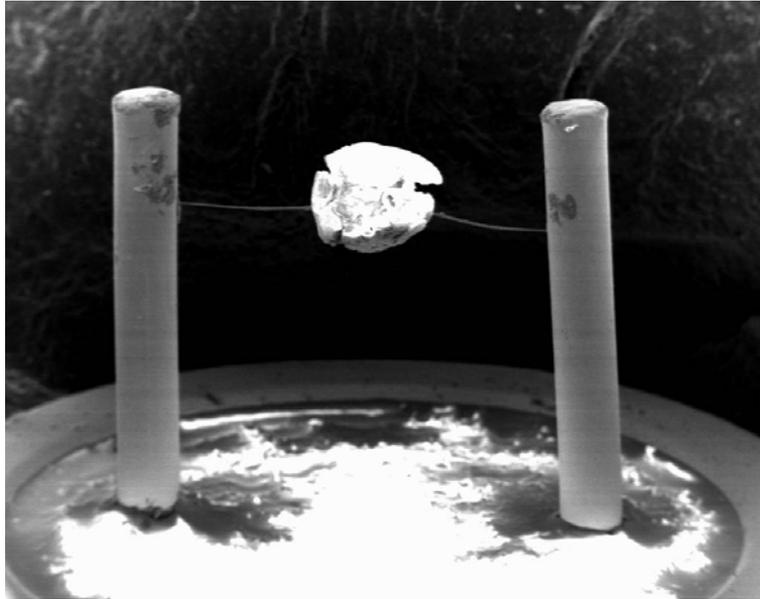
**Figure 2 - Scanning Electron Microscope Photograph Of The Pellistor Bead**
