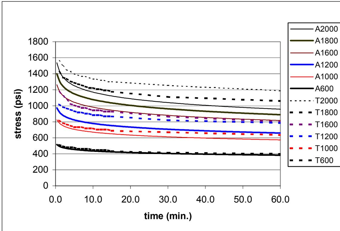
**Figure 11 - Stress Experimental Results (T) Compared to ANSYS Stress Relaxation Solutions (A)**
