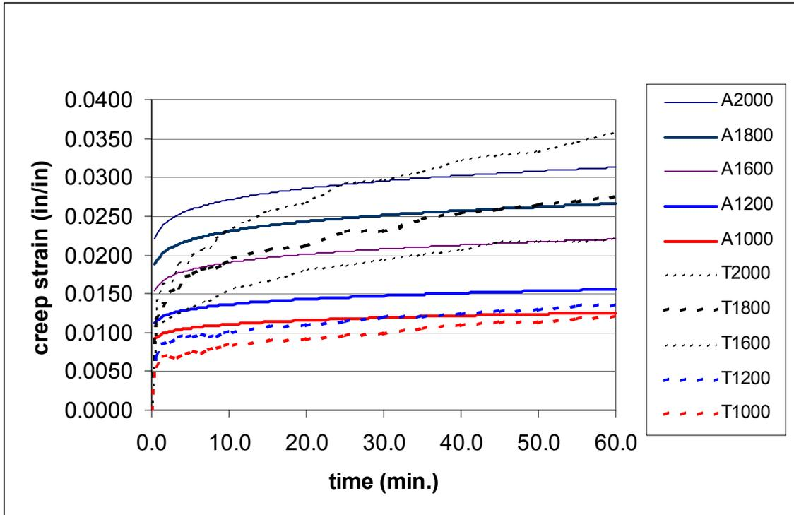
**Figure 10 - Creep Experimental Results (T) Compared to ANSYS Adjusted Creep Solutions (A)**
