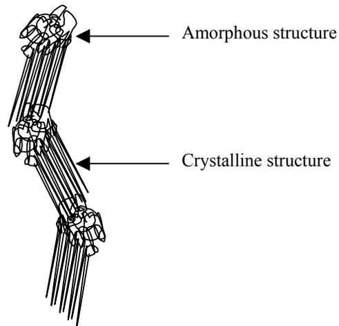
**Figure 1 - Schematic of Polypropylene Molecule Structure**
