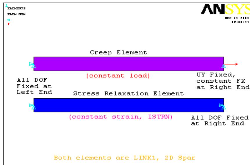
Figure 8 - ANSYS Models for Stress Relaxation and Creep
