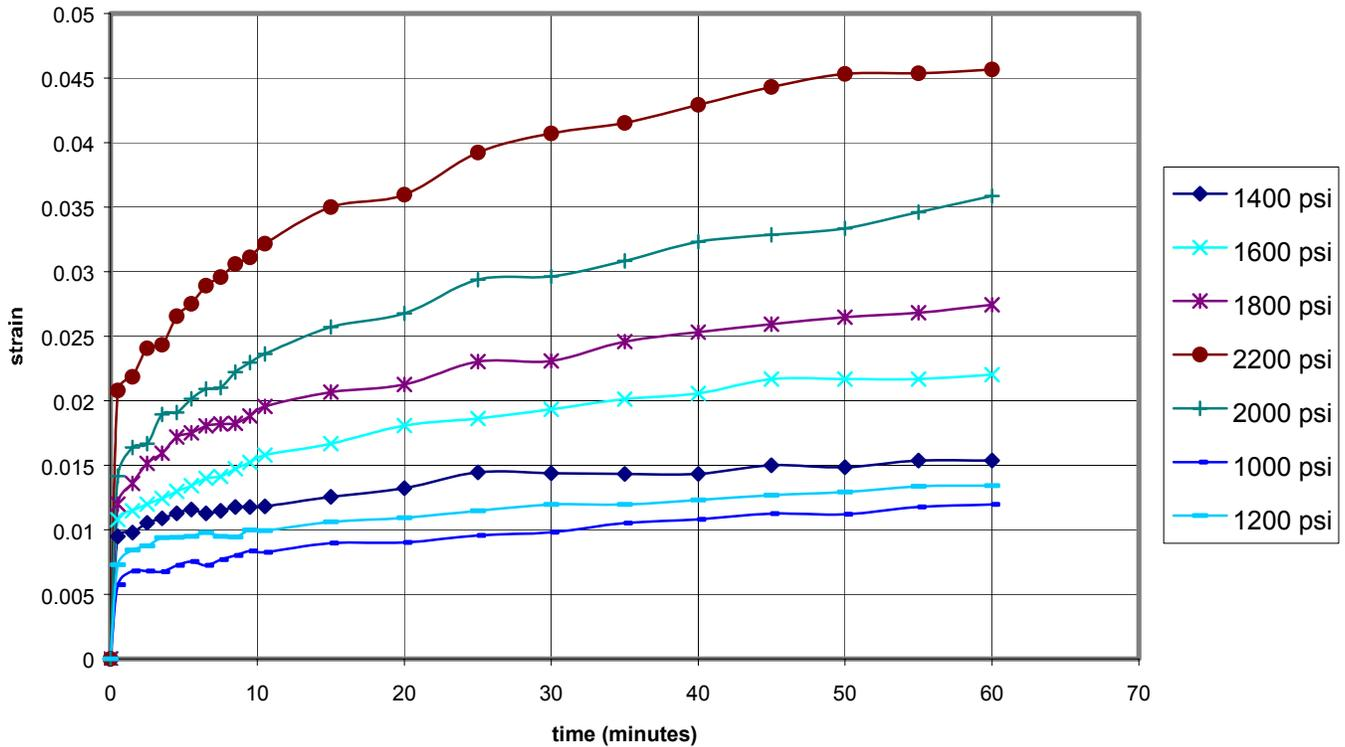
**Figure 5 - Polypropylene Creep Experimental Results: Strain versus Time for Family of Stresses**
