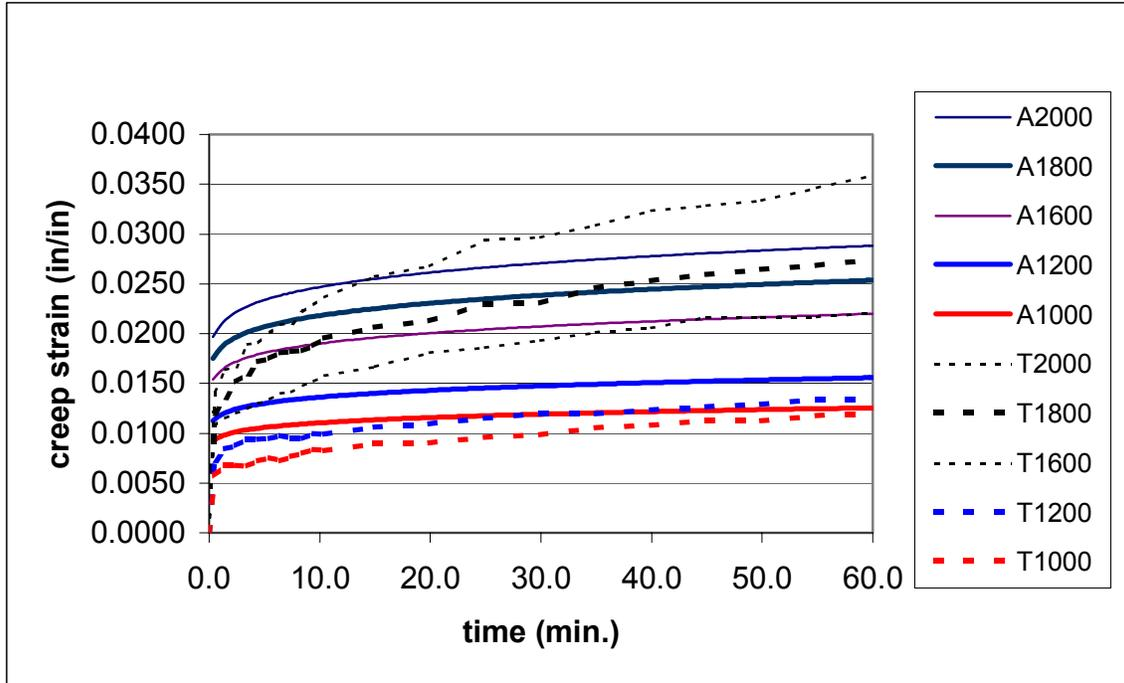
**Figure 9 - Creep Experimental Results (T) Compared to ANSYS Creep Solution (A)**
