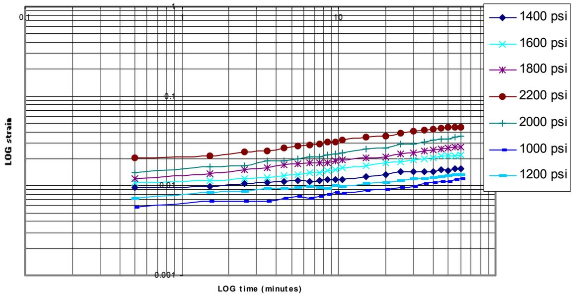
**Figure 6 - Polypropylene Creep Experimental Results: log Strain versus log Time**
