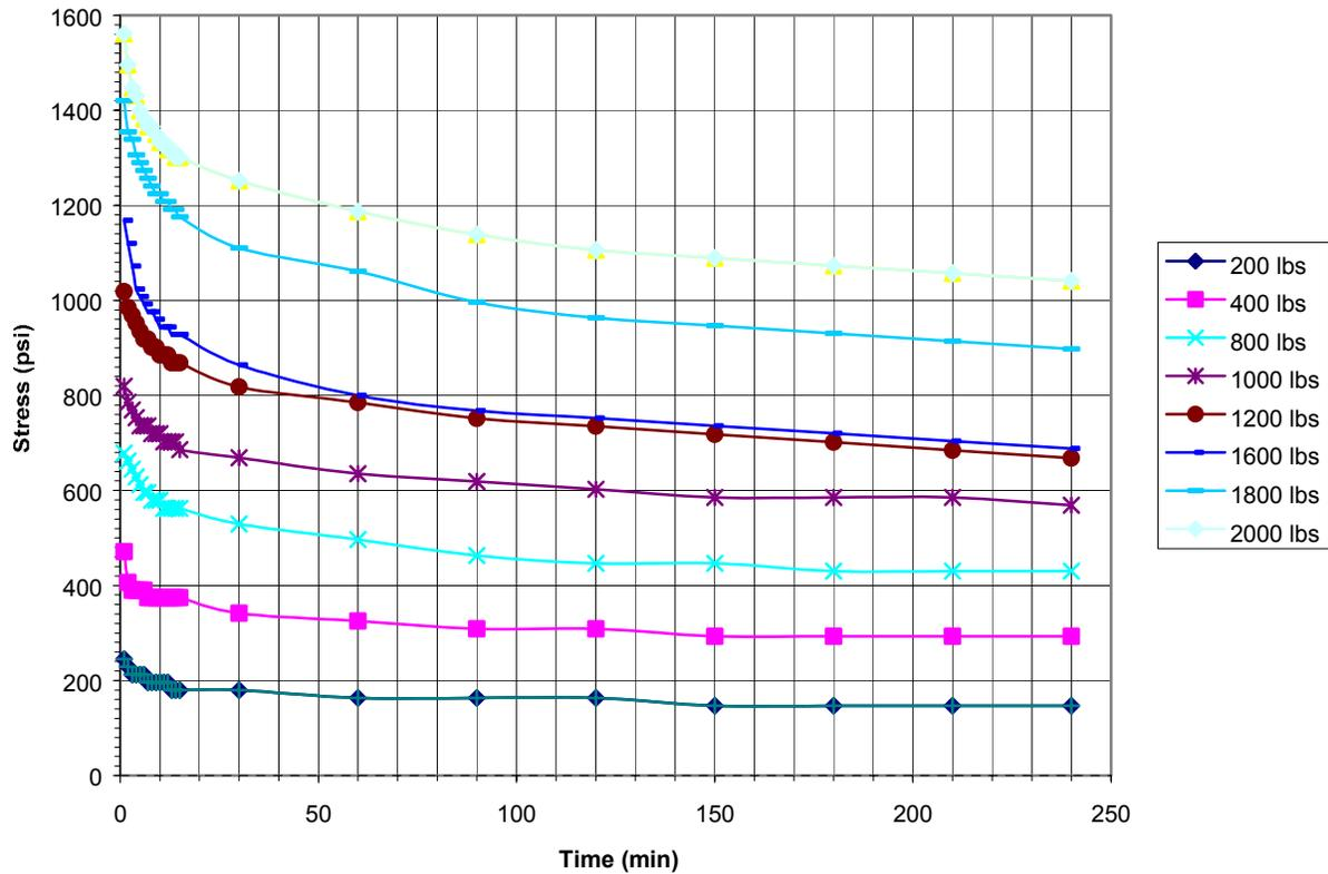
**Figure 3 - Stress Relaxation Response of Polypropylene To Family of Stresses**
