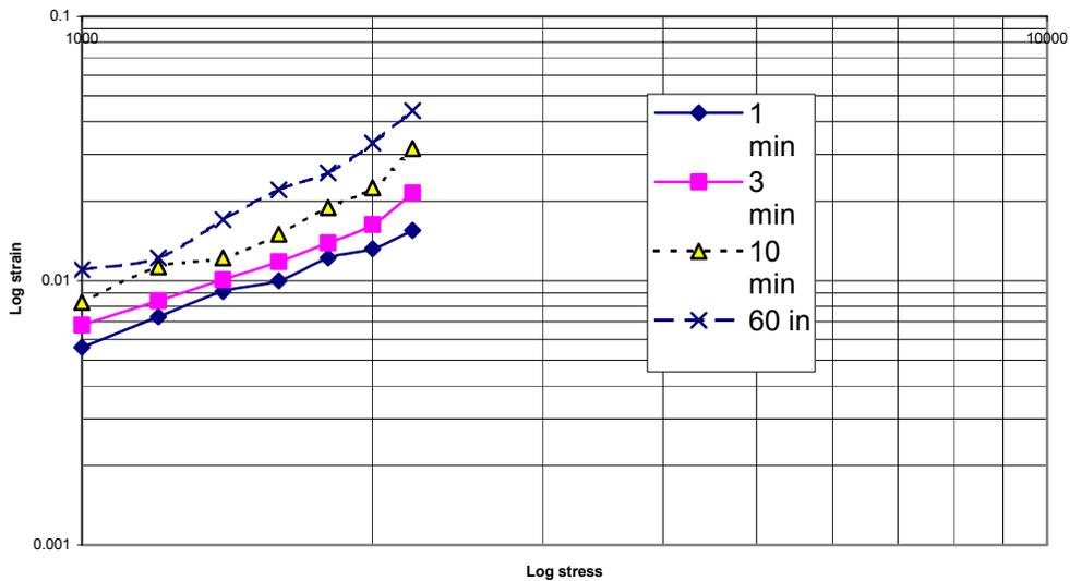
**Figure 7 - Polypropylene Creep Experimental Results: log Strain versus log Stress**
