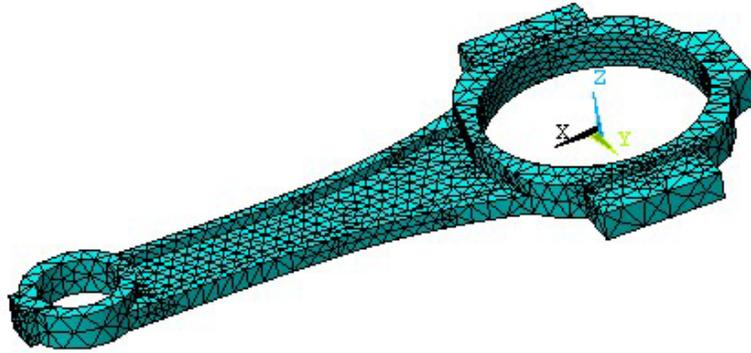
**Figure 4 - Connecting rod finite element model**
