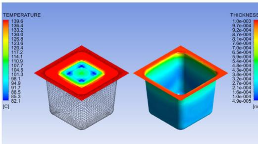
Optimized temperature profile (left) and resulting wall thickness distribution (right) for a simple test cup.
