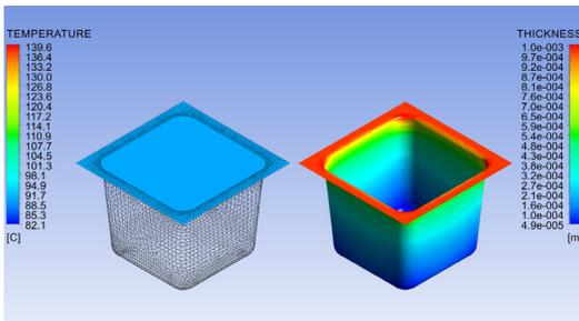
Homogeneous temperature profile (left) and resulting wall thickness distribution (right) for a simple test cup.
