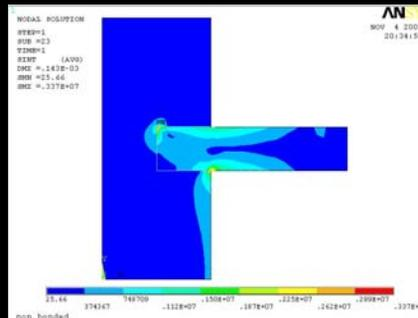
*Cantilever beam models were used to determine stresses in teeth, socket and gum tissue resulting from impact.*
