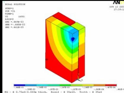
*The cushioning effect of the soft layer of the mouthguard was analyzed with an explicit finite element code to predict impact force given the geometry, material properties and impact velocity.*
