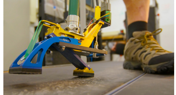
HuMoTech’s prosthetic foot worn by a user with unilateral transtibial amputation.
