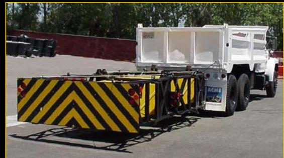
Energy-absorbing aluminum baffles in the hinged truck-mounted attenuator serve as crash cushions.
