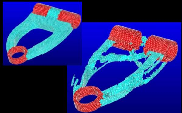
Starting with an initial mesh (left), the ANSYS topology optimization routine automatically eliminates elements with stiffness below a specified threshold (right). The result is an analysis model consisting only of the elements needed to maintain the required stiffness with minimal material (patent pending design).
