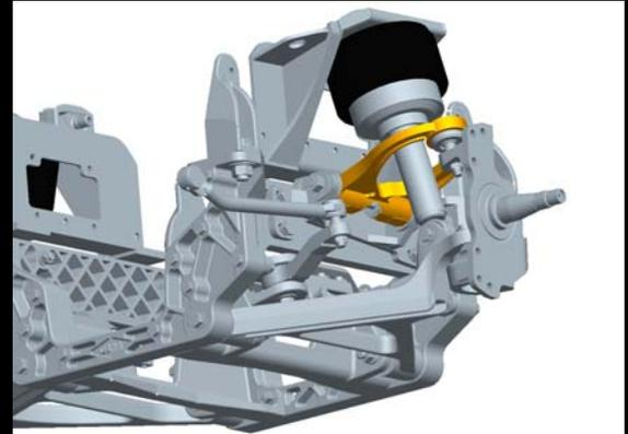
Designed by Dana Corporation for commercial vehicles, the upper control arm (highlighted) is a critical component in the front suspension system (Dana patents pending).
