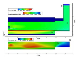
The contour of heat flux and temperature distribution in the IRSI indirect pyrolysis system. The volatile gas derived from the biomass material burns in the combustor to produce significant percentage of the heat required for thermal conversion (Energy, Vol. 169, pp. 1101-1111, 2019).
