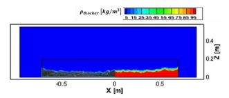
The schematic of the real biochar produced by IRSI (left side) and the simulation contour (right side). The red represents biochar density. The simulation was performed with Ansys Fluent, in a study conducted by the University of Alberta and the University of Vigo.
