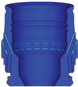
Casing hanger cumulative damage distribution
