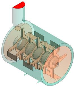
SBP reactor domain (half-symmetric) for the base case with two nozzle inlets
