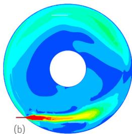
Velocity distribution cross-section for (a) the base case with two nozzles, and (b) a modified setup with four nozzles
