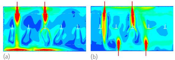
Flow pattern on a plane cutting across the injection nozzles for (a) base case with two nozzles (b) modified setup with four nozzles
