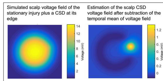
In the left panel, the stationary voltage field representing a residual voltage caused by the injury to the brain is combined with the voltage field of a CSD, obtained using ANSYS simulation. The CSD signal is just barely visible as a very slight bump at “2:30 o’clock”. In the right panel, the CSD voltage field becomes fully visible after subtraction of the temporal mean of the complete voltage field.
