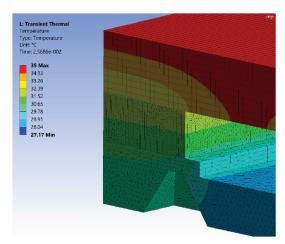
Results from a transient thermal simulation. The simulated transient temperature distribution can in turn be used to improve the design.
