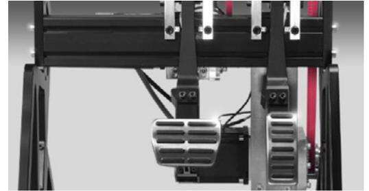
With this module, you can control professional haptic steering wheels and pedal force feedback hardware. From the GUI, you can easily parametrize the steering wheel and pedal controls (stiffness, damping, maximal torque, friction, etc.), as well as additional vibration (depending on road type).
