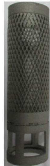
Figure 1: Filter produced by Croft Filters showing bulge on what should have been straight walls.
