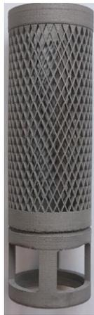
Figure 7: Physical build of 1.0 magnitude distortion compensated file showing no external bulge and nearly vertical walls.
