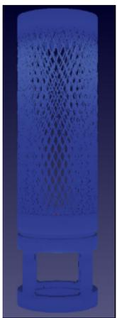
Figure 6: Simulation results of two iterations of distortion compensation at a factor of 0.5.
