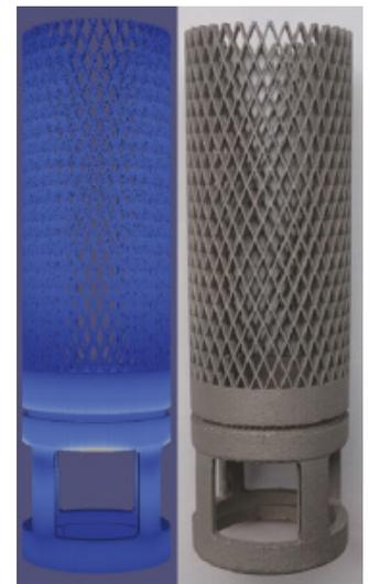
Figure 2: Simulation and physical build images showing no bulge before top ring is added.
