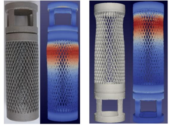
Figure 4: Simulation accurately predicted that the bulge in an inverted filter will occur in a different portion of the mesh region, just below ring.
