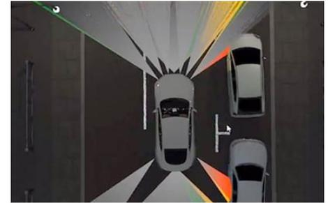
You will benefit from powerful ray-tracing capabilities to recreate sensor behavior and be able to easily retrieve sensor results through a dedicated interface. This solution provides a unique way to collect virtual sensor information during real-time drives and use the information to develop autopilot code.
