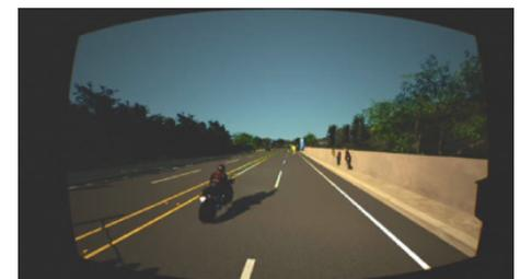
The camera simulation creates raw images, which are used to test and validate perception algorithms either as models (model-in-the-loop) or software (software-in-the-loop).
