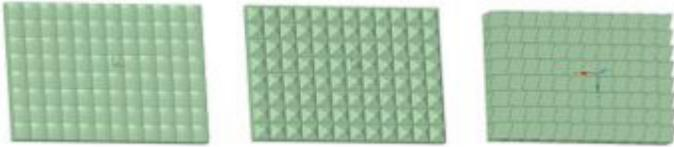
Optical lenses can use any freeform support, which can be split into smaller elements to achieve the intended style. Different types of grid patterns are available: rectangular, circular, stripe or freestyle using design input directly.
