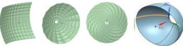
Ansys SPEOS Optical Part Design has an advanced mode for the sharp cut-off definition. Using this mode, an expert can design better lighting distribution based on the definition of control points, control horizontal and vertical beam distribution, and progressive tilt. This simplified process provides greater flexibility on the beam definition for better performance on the road. A viewer displays the optical beam pattern or relative photometry on an intensity grid for any selected face.
