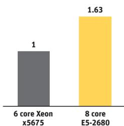
Intel Xeon® E5 processors have demonstrated a 63 percent performance increase on the geometric mean of 10 ANSYS Mechanical™ benchmarks over the prior Xeon 5600 family.
