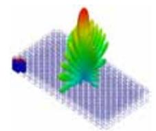
Distributed memory enabled efficient electromagnetic simulation of this 256-element skewed waveguide array using ANSYS electromagnetics tools.
