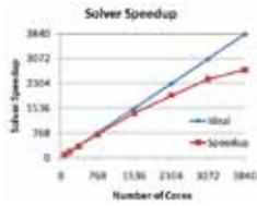
The largest CFD benchmarks from ANSYS yield nearly linear scaling up to 3,072 processors, reducing turnaround time from hours or days to just minutes.
