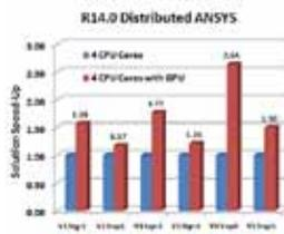
GPU computing supports distributed memory structural solutions in the latest ANSYS software, yielding single-machine speed increases of up to two times over a range of benchmark problems.
