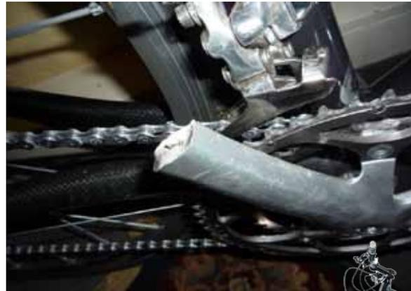
Bicycle crank shaft broken due to fatigue
