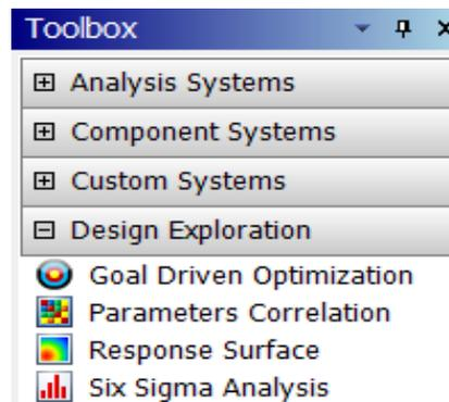
You can add design exploration systems to the ANSYS Workbench schematic — which can then be applied to all physics — with drag-and-drop simplicity.
