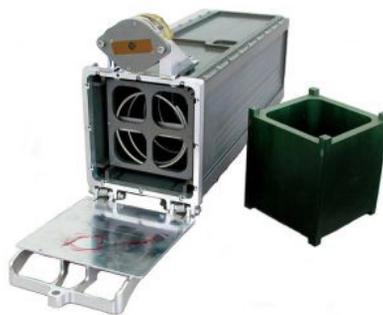
Modal analysis for Cornell's nanosatellite ensured that the structural walls provide adequate stiffness during launch.
