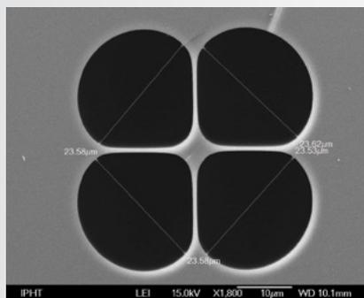
Microstructures in silica fiber and response to external stress
