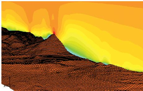
Velocity contours on a plane slicing through the highest peak in the landscape show a variety of wind speeds near ground level
