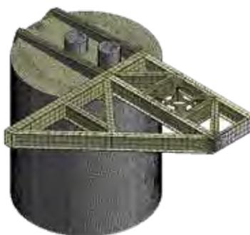
Finite element mesh of a suction pile
