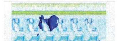
Inspired by recent headlines about the spread of airborne infectious diseases, Raymond Wang, 17, used ANSYS CFD to model an aircraft cabin and simulate how pathogens spread via cabin airflow. He then used that information to design an air inlet director system that increases the quality of air for each passenger. For this study, Wang won a cash prize and the Gordon E. Moore Award at the Intel International Science and Engineering Fair.
