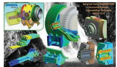
▲ Simulation of a spherical valve for a hydroelectric plant inlet. ANDRITZ Hydro, whose entry was named to the Hall of Fame, reduced the weight of the valve inlet with the help of simulation.
