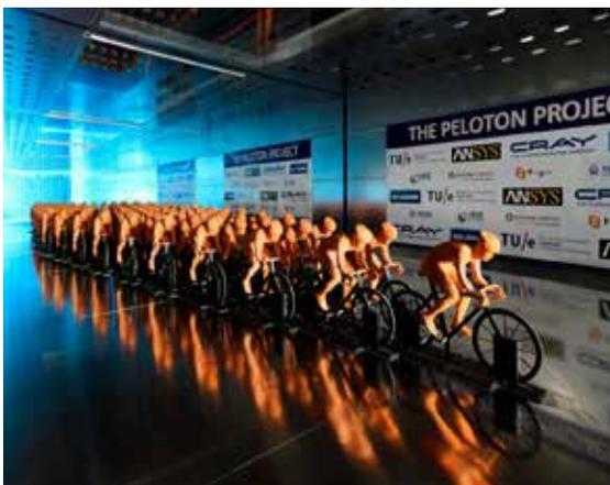
Fluent simulation on a Cray computer to find out. By determining the flow pattern between each cyclist in the peloton, the team found that the riders at the core of the peloton experience much less drag than was previously expected. This was the largest CFD model ever performed for sports.
