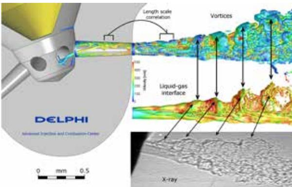
Delphi Automotive Systems used ANSYS simulation to explore vortex-driven atomization in high-pressure diesel injection.
