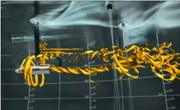
To capture energy from ocean tides to create renewable energy, researchers at Cardiff University used ANSYS simulation software to analyze wakes captured by tidal stream turbines to increase reliability and reduce costs of tidal energy.
