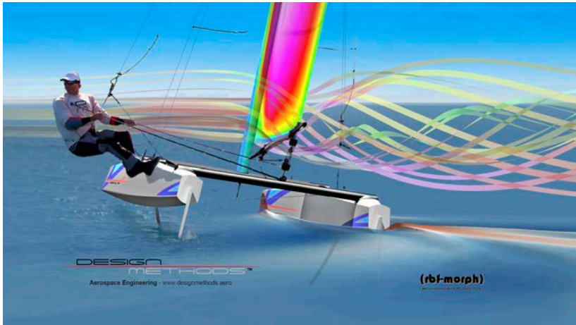
▲ Design Methods coupled ANSYS Fluent for aerodynamic analysis to rbf-morph to successfully design an A-class catamaran sail.
