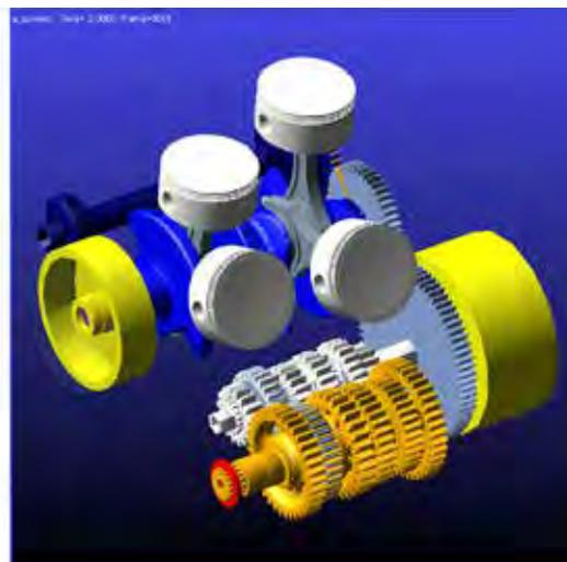
ANSYS Workbench fretting fatigue study helped determine component wear damage by simulating the exchange of forces between the conrod and the crankshaft while the engine is running.
