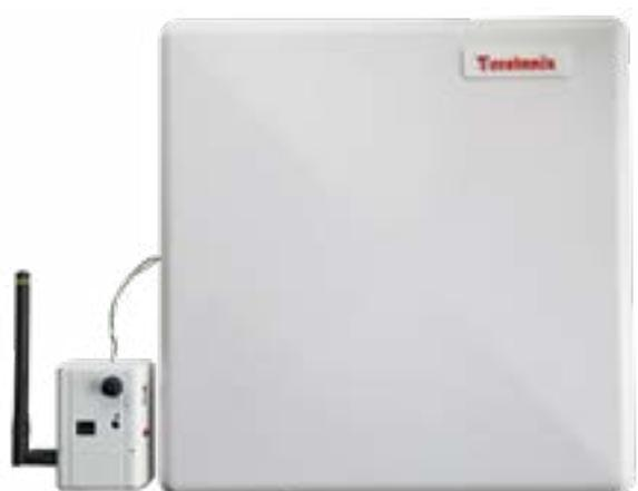
**Prototype of an industrial IoT sensor node. Multiple sensors, a microprocessor and a wireless data transmitter/receiver are powered by the Teratonix ambient RF harvester, composed of an antenna, RF-to-DC converter integrated circuit, and DC regulation and storage circuit.**
