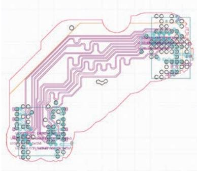
▲ Extracted subset of Allegro layout including memory chip, controller and traces, and assigned ports used to model data byte 0 in Designer-SI.
