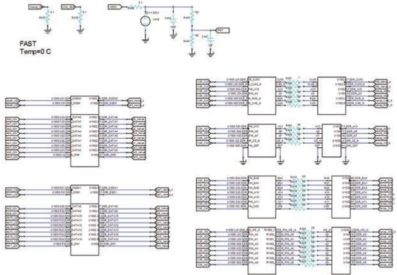
▲ Schematic page for simulation (top). All extracted trace models are placed here and connected to package and buffer models. Each box is an HFSS model of DDR3 traces.
