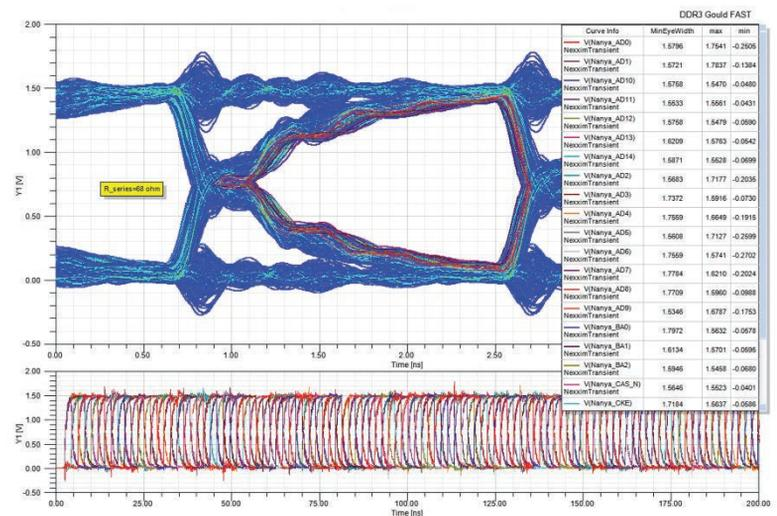
▲ Single-ended DDR3 address and control signals with 68 ohm resistor termination. With this value, the design passed AC overshoot and undershoot specifications.
