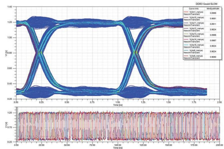
▲ Eye diagram of data signal with 60 ohm internal termination
