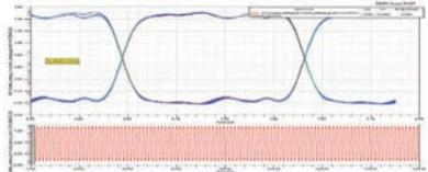
▲ Differential clock eye diagram without series termination
